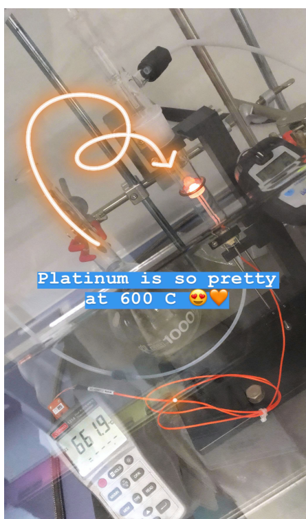
Figure 3.1: Image of the annealing setup at DESY 2019 with commentary about the color of platinum at the temperature shown. Here the coil of the induction furnace can be seen wrapped around quartz tubing in which the platinum crystal is encased. 100% CO gas is being flowed around the crystal, and the temperature is being roughly monitored by a digital thermometer attached to the quartz that is holding the crystal.
