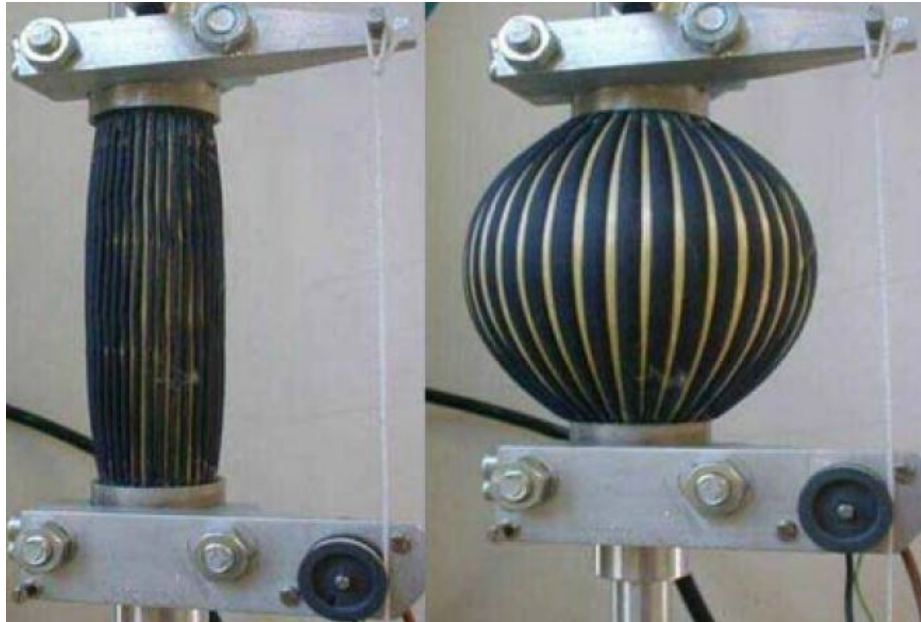
Figure 1.7: Schematic of deflated and inflated state of the Pleated Artificial Muscle [83].
