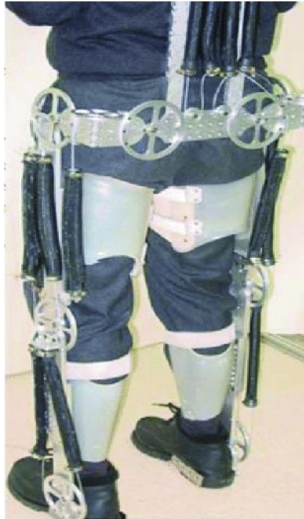
Figure 4.2: Schematic of a 10-DOF exoskeleton robot with PAMs utilizing PID control strategy [15].
