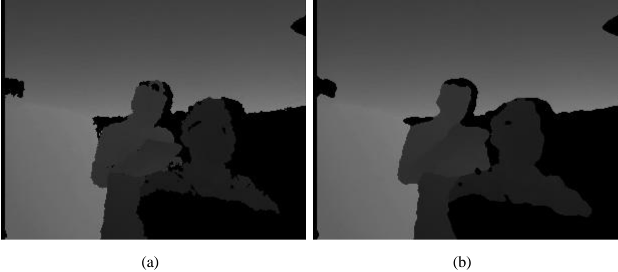
Figure 3.10 Denoising of depth images: (a) original depth image; (b) depth image after denoising.
