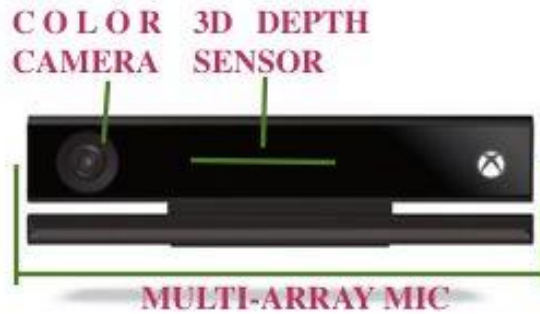
Figure 3.2 Overall hardware specifications of Kinect Xbox One sensor [89].
