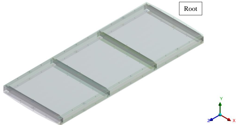
Figure 16 – The 92 Fastening Points / Longitudinal Spring locations (Blue dots) [19]
