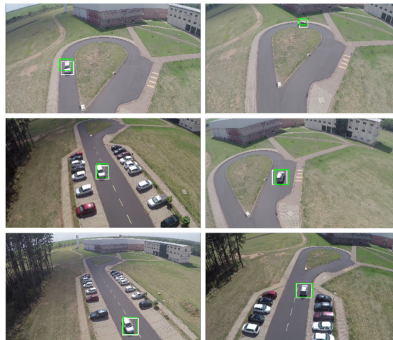
Figure 22 – Test Vehicle Tracking: Box green see our LSTM track and the white box is the real box (Video#1).
