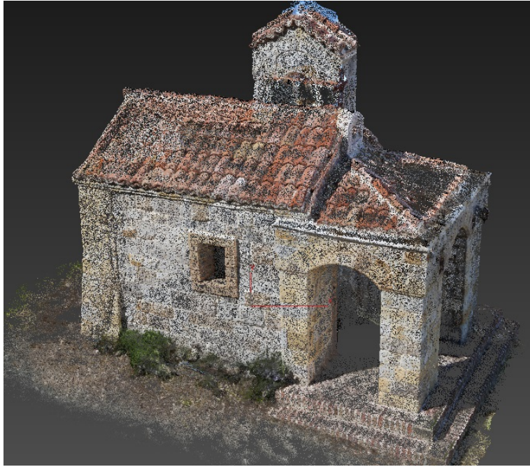
FIGURE 2.1: Example of a raw point cloud with colour values for each point, captured with a LiDAR scanner. Adopted from Autodesk tutorial 1 .
