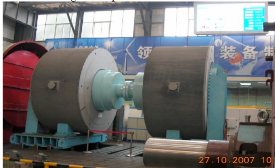
Figure 3-4: The prototyped 2MW DD RF-PMSG used as a benchmark [16]
