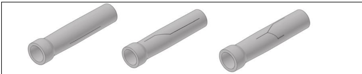
Figure 2-3 - Longitudinal cracks (Rodriguez et al, 2014)
