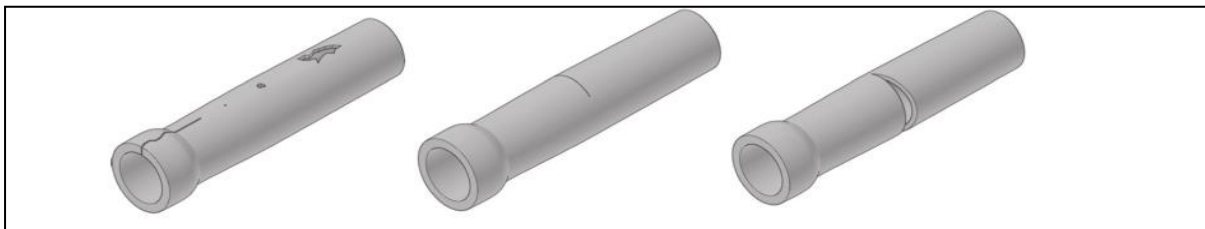
Figure 2-4 - Circumferential cracks and round holes (Rodriguez et al, 2014)
