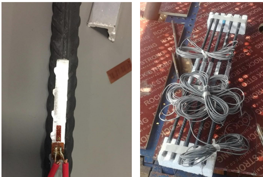
Figure 52 Manufacture of rebar mounted foil type strain gauges
