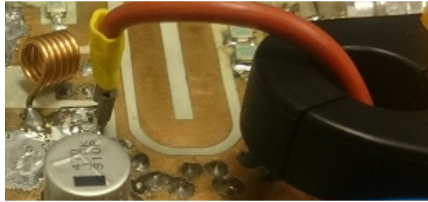
Fig. 16: Current sensor used to measure the drain current.
