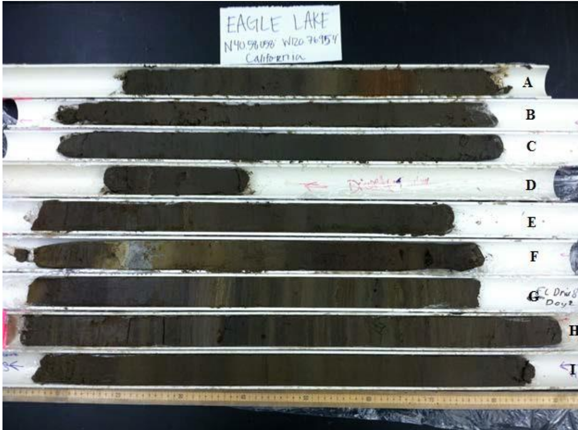
FIGURE 11. Photograph of ELSB11. Drive A is the youngest and I is the oldest. Stratigraphic up is to the left for each drive. Multi-proxy analyses were done on ELSB11-D1 (A), ELSB11-D2 (B), ELSB11-D7 – D10 (F-I). The late Holocene section is represented by cores A and B and the early Holocene section is represented by cores F – I. Mazama ash can be seen in the ELSB11-D7 (F) as a dark gray layer. Laminations can be seen in the second half of core ELSB11-D8 (G) and all of ELSB11-D9 (H).
