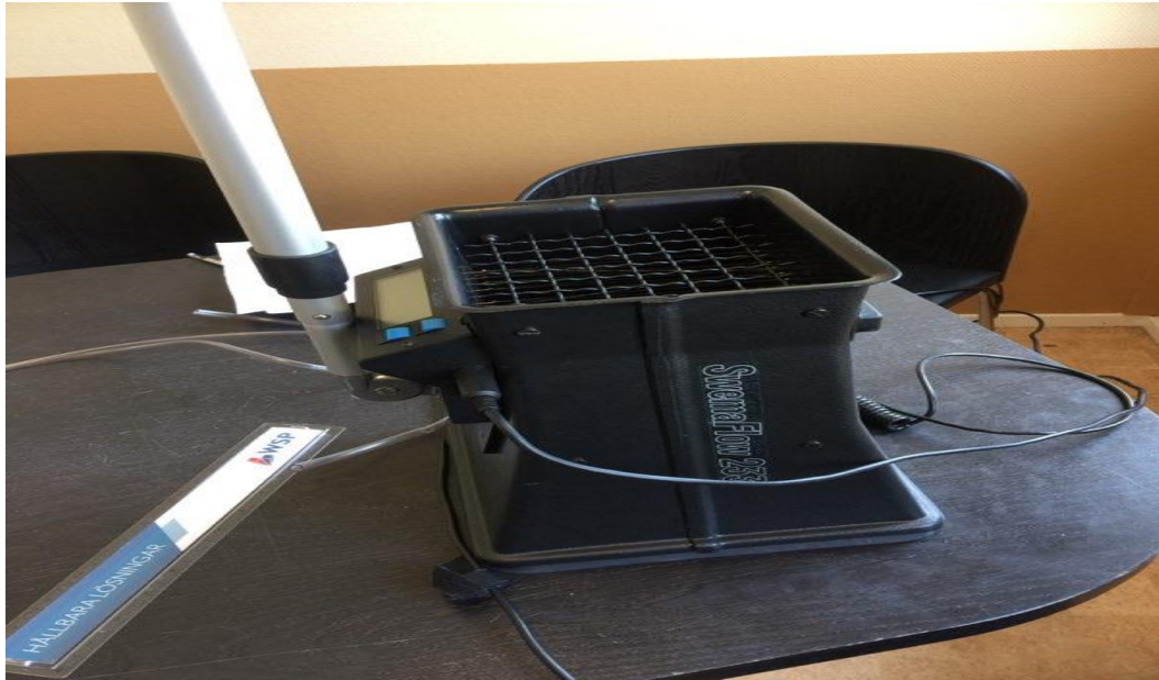
Figure 3-2: Airflow meter for measuring airflow rate.
