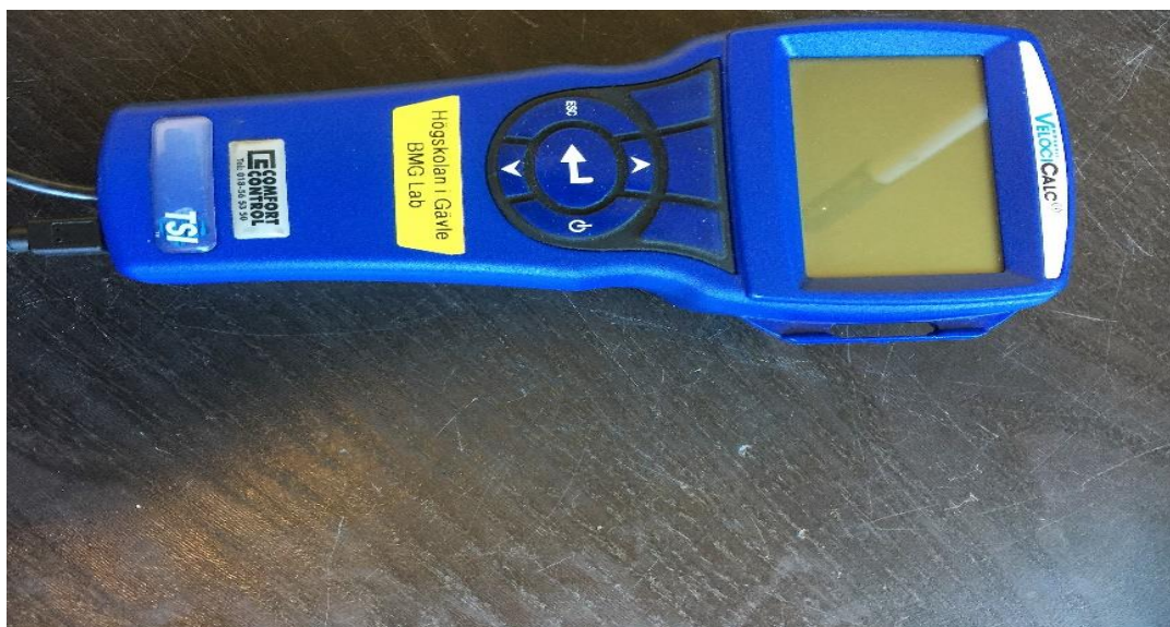
Figure 3-1: Anemometer for measuring air velocity meter and volumetric flowrate.
