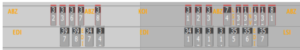
Figure 7: Example of schedule with carry in and carry out concept where ABZ is a base. The rectangles represent flights and the numbers inside them represent the tail number. The three letter codes represent the airports.
