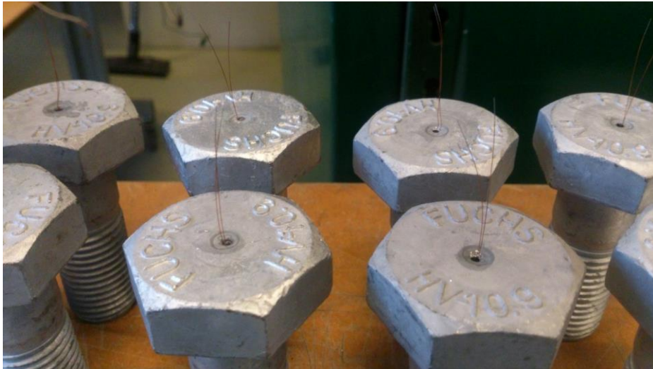
Figure 26 Bolts with strain gauges glued inside the holes.
