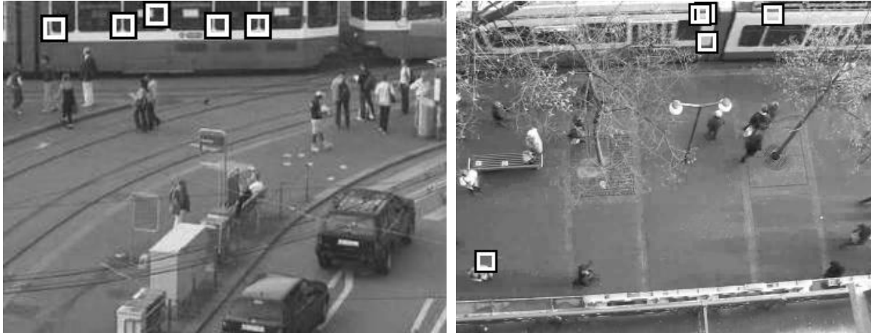
Figure 4.33. Two scenes exemplifying the motion tracking model used for visual saliency calculation, and visual attention selection of the 5 strongest targets. Many of the targets correspond to the moving trains in the background, which is not as useful for target selection.
