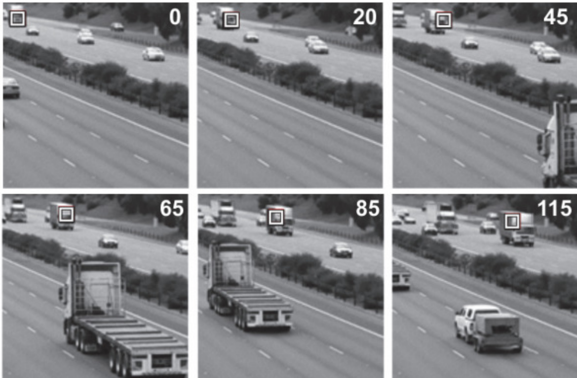
Figure 4.25. Selected frames of the network tracking a truck in highway video footage with the frame number listed in the top-right corner. The gaze generated by the tracking RBM is represented by the black and white square.
