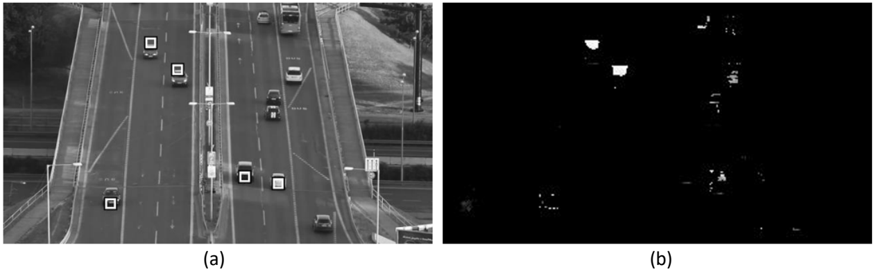
Figure 4.32. (a) Visual attention selection of the 5 strongest targets denoted by the black and white squares based on (b) the motion tracking model’s visual saliency calculation. Each of the targets corresponds to separate moving vehicles.
