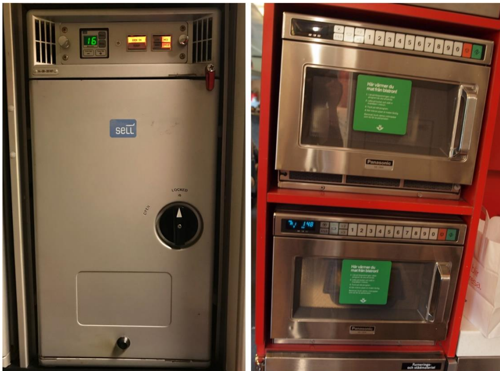
Figure 6. Left: an integrated oven in a Boeing 747 commercial aircraft. Right: two microwave ovens on a commercial train in Sweden.
