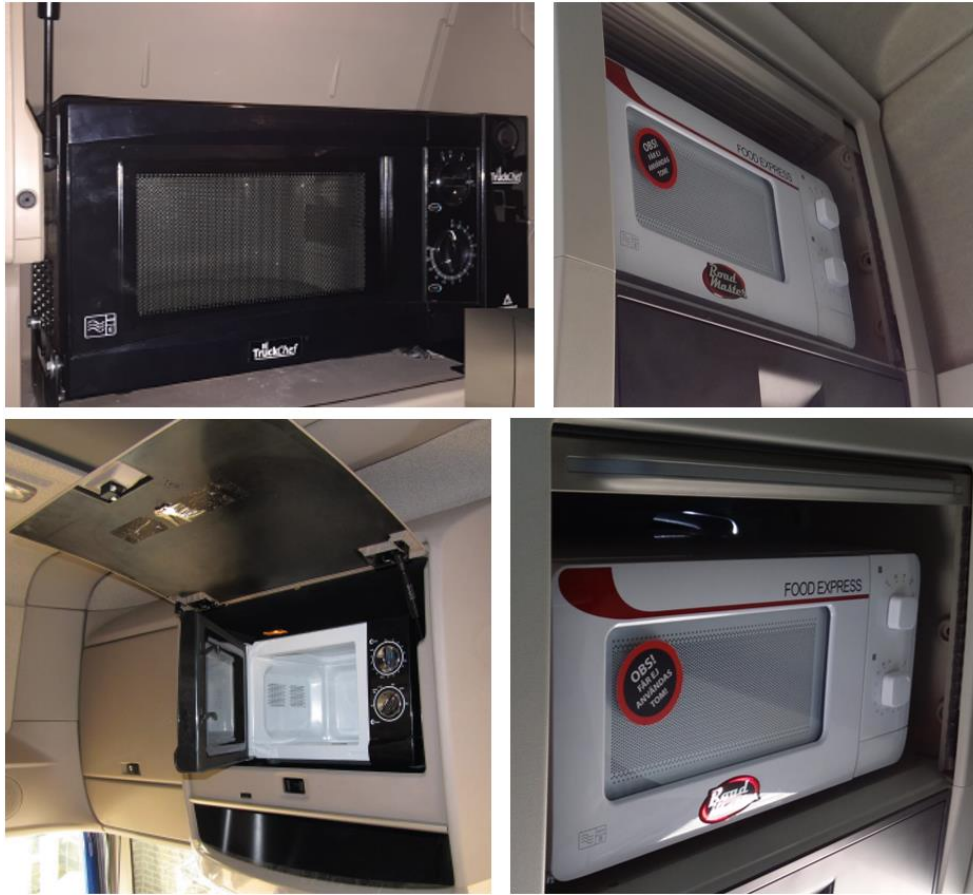
Figure 5, a collage of truck cabin integrated microwave ovens kept behind a jalousie or shutter.
