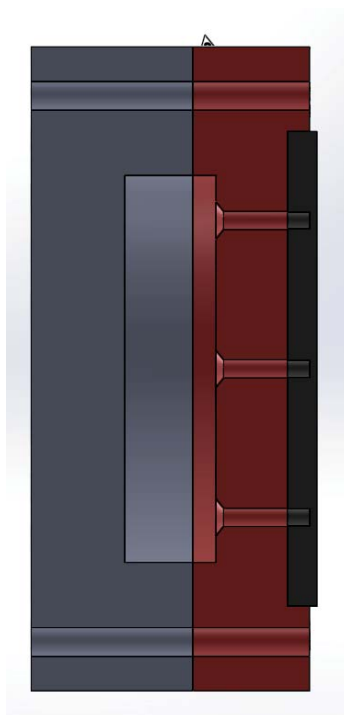
Fig. D.5.: Wear plate and Pre-chamber cross section drawing
