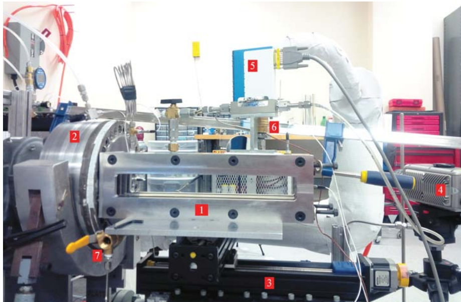
Fig. 2.1.: Combustion chamber (1) sitting on XY positioning table (3) while facing the pre-chamber (2). A C-clamp (6) holds it firmly in place. Also shown are air inlet (6) and outlet (7) for main chamber heating and mass flow controller (5) for fuel delivery and a High speed camera (4).
