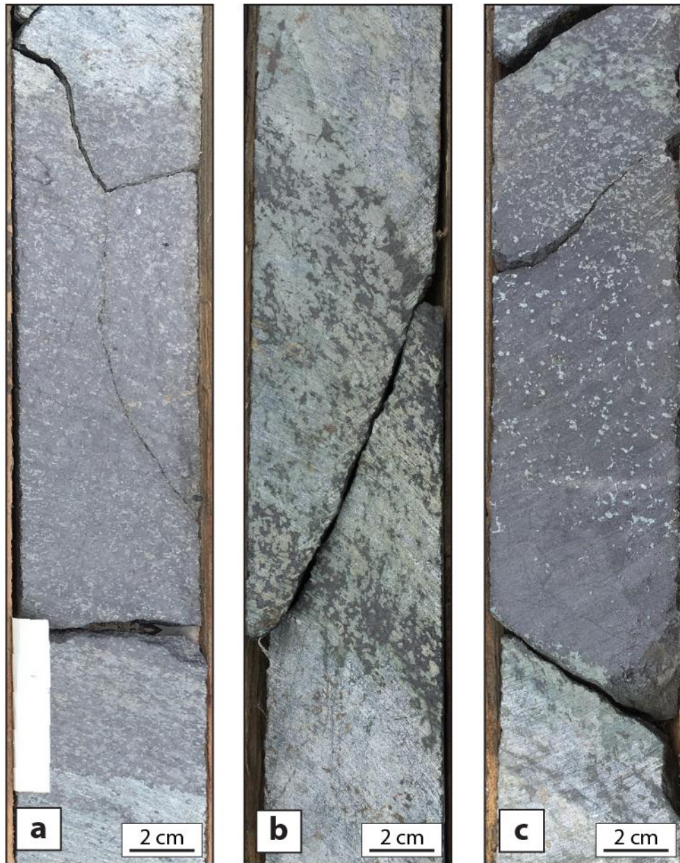
Fig. 5. Photos of representative oxide-rich lithologies and layering textures observed in drill cores. a. Homogeneous magnetite-rich olivine pyroxenite layer with sharp upper and lower contacts with adjacent leucogabbros, MA-09-11, ~40.7 m drill core depth; b. Magnetite-rich metagabbro layer with sharp upper and lower contacts with neighbouring leucogabbros, MA-10-32, ~76.6 m drill core depth; c. Massive oxide layer with normally graded Fe-Ti oxides. Note the sharp basal contact with underlying leucogabbro with alteration rim of amphiboles, MA-10-32, ~78.2 m drill core depth.
