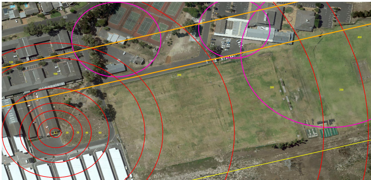
Figure 7.11 Cellular transmitter and HVAC power lines EMF radiation exposure intersecting with tennis courts, library, sports field and community centre.
