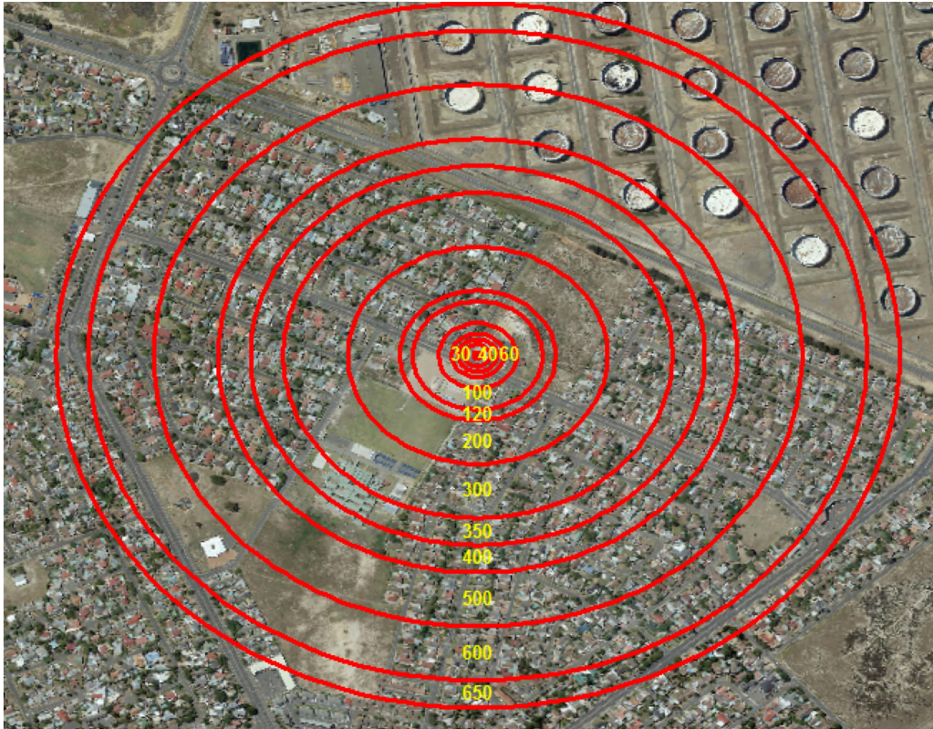
Figure 7.7 Multiple ring buffer analysis feature class of cellular RF-EMF radiation compliance distance from Table 6
