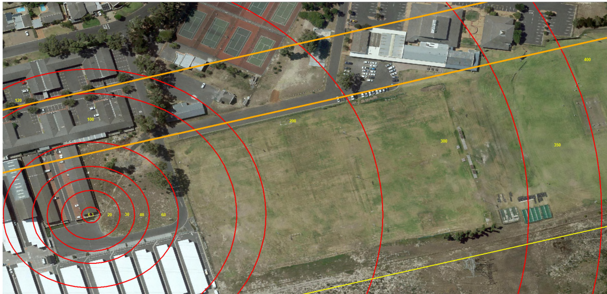
Figure 7.8 Multiple ring buffer analysis feature classes of ELF and RF-EMF radiation compliance distances
