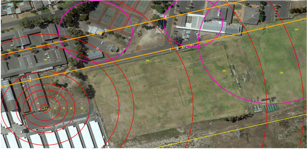
Figure 7.10 Cellular transmitter and HVAC power lines EMF radiation exposure intersecting with tennis courts, library, sports field and community center.
