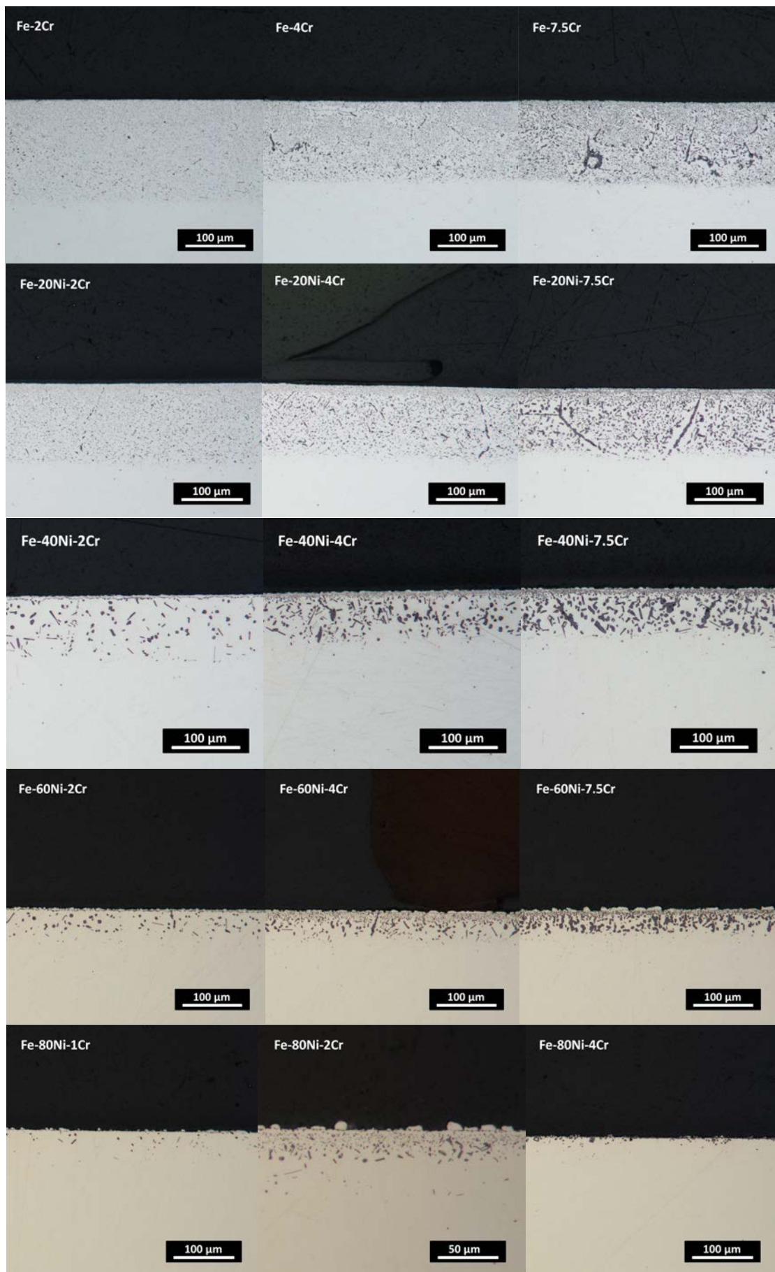
Figure 4.11: Micrographs of IOZ after exposure in H 2 /H 2 O gas with 13% water vapour at 1,000°C for 150h.
