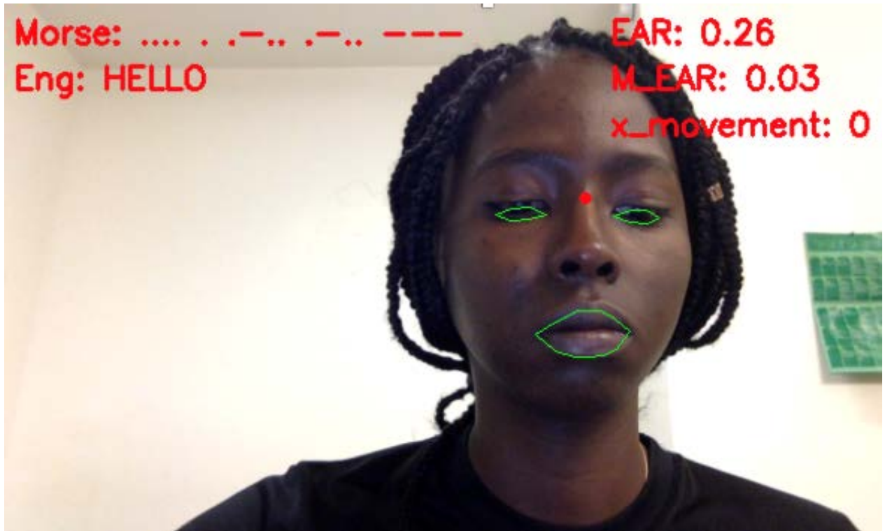
Figure 4.22: Depiction of the system being used to spell out "Hello"
