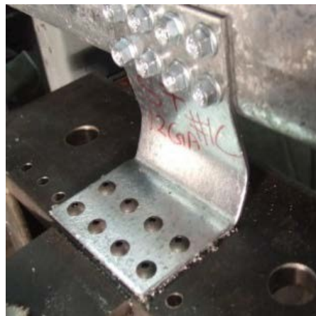
Figure 2.4: Failure modes of clip angle in compression
