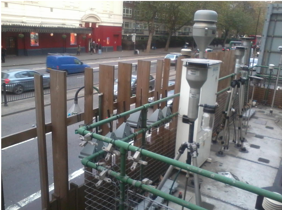
Figure 2.2 Six AQMesh pods attached to the pipe railing using cable ties. Reprinted with permission from Barratt, B. (235)
