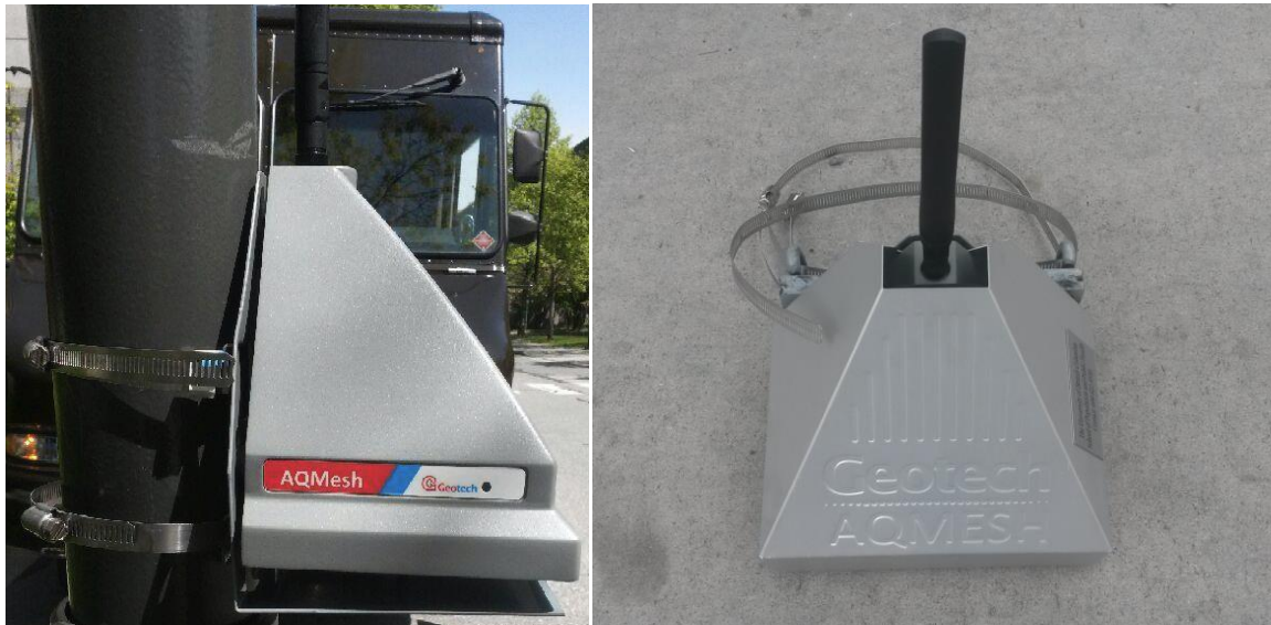
Figure 2.1 AQMesh unit (left) equipped with the solar shield and the pipe clamps (right)
