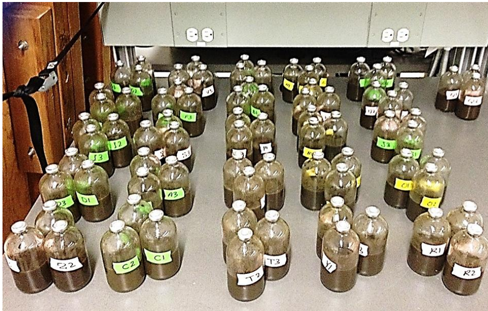
Figure 4-3. The photo of the batch anaerobic digesters
