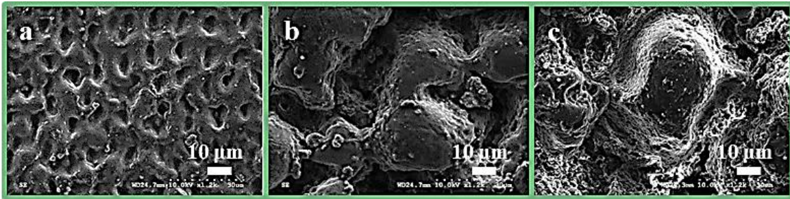
Figure 6.8. SEM pictures of imprinted medical-PVC replicated from femtosecond laser ablated SS, a) Paraboloidal, b)Tripled, and c) Cauliflowered patterns
