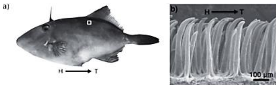
Figure 6.12. a) Picture of filefish N. septentrionalis , b) The SEM picture of the superoleophobic skin of the fish; arrow directing from head (H) to tail (T) indicates the oriented direction of hook-like spines (image adopted from reference [50] with permission)
