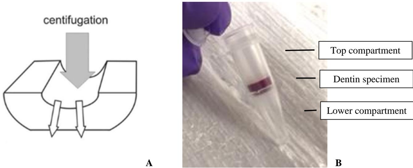
**Figure 5 Mode of centrifugation. A) The side view of a dentin block is shown; the root canal is visible in the middle. With the power of centrifugation the bacterial suspension is forced into the dentinal tubules. B) A Nanosep microfiltration tube is shown with a dentin specimen in place; the top compartment is filled with the bacterial suspension prior to centrifugation. The bacterial suspension is collected in the lower compartment after centrifugation. (83)**
