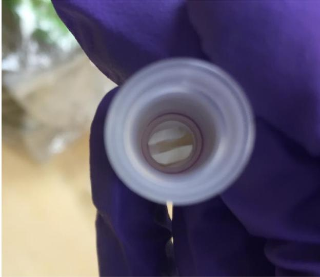
**Figure 4 Specimen placement inside Nanosep filter tube prior to gap sealing**
