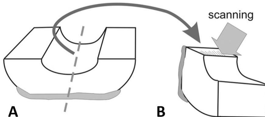
**Figure 8 Fractured specimens indicating the exposed area for confocal laser scanning microscopy (CLSM) (83). A) Dentin block after experimental procedures; the backside of the specimen is covered with nail varnish. B) The dentin block is sectioned through the center of the root canal; the longitudinal dentinal tubules are exposed and can be viability stained prior to CLSM.**
