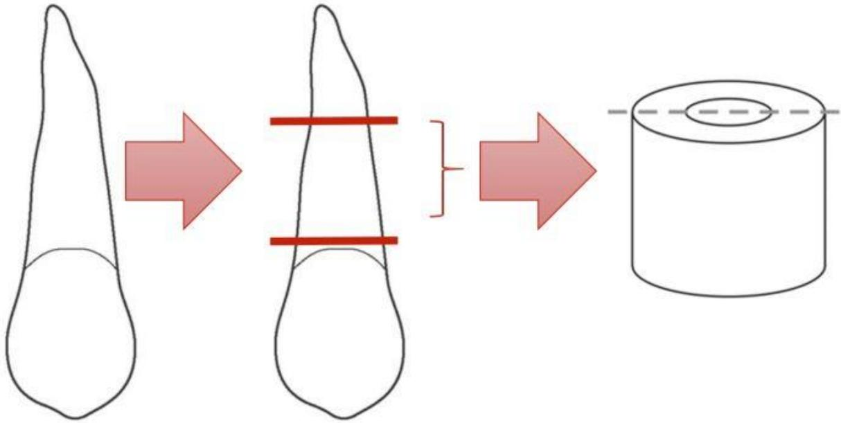
**Figure 2 Schematic drawing of a cylindrical dentin block. The coronal part of a single-rooted tooth is used to create samples. (Courtesy of Ma et al 2011)**
