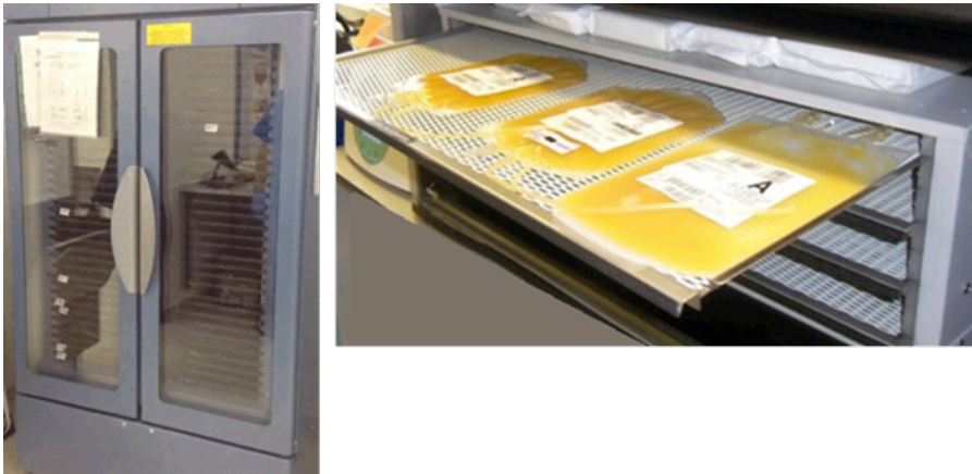
Figure 1.3 Storage of platelet bags in blood banks. Platelet storage bags are stored in platelet incubators at 22 °C on agitators that provide side-to-side motion.
