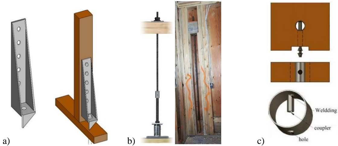
Figure 4.1 Hold-downs for timber structures: a) Traditional option; b) Strong-Rod™ (Simpson Strong-Tie Ltd.); c) Tube connector (Schneider et al., 2014)
