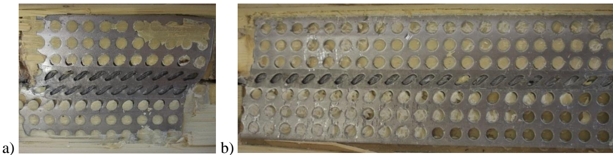
Figure 4.12 Failure mechanism: a) Two rows covered; b) One row covered
