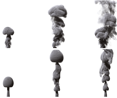
Figure 3.6: Two sequences from 3D rising smoke simulations. Top row: MC-IVOCK with vortex stretching. Bottom row: MC-IVOCK with vortex stretching switched off. With vortex stretching, vortex rings change their radius under the influence of other vortex rings, these process can easily perturb the shape of vortex rings, breaking them to form new vortex structures, which brings rich turbulence into the flow field.
