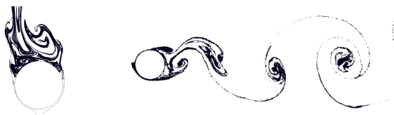
Figure 2.3: Our method captures the velocity field near the boundary efficiently and with high apparent fidelity. Left: zoom-in near the boundary flow. Right: the entire simulation, \text{Re}=15000 .
