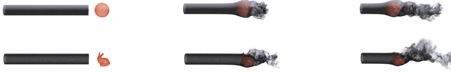
Figure 4.12: Moving objects in slightly viscous flow generate turbulent wakes. Top row: vortex shedding from a moving ball. Bottom row: a moving bunny.
