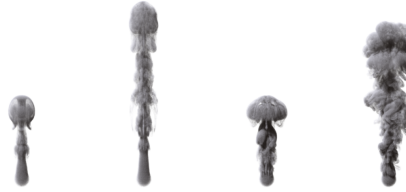
Figure 3.12: IVOCK can be cheaper and higher quality then taking small time steps. Left and mid-left: BFECC. Mid-right and right: BFECC-IVOCK with twice as large a time step, computed in much less time.
