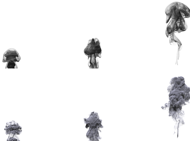
Figure 4.11: Comparison of VIC and PPPM. Top row, sequence of 64^3 VIC simulation; bottom row: PPPM using the same resolution grid. Notice that the large scale motion of the two simulation matches before the point where turbulent motion becomes dominant.
