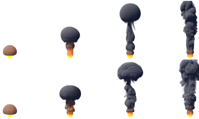
Figure 3.15: Fire simulations making use of our combustion model. Top row: BFECC. Bottom row: BFECC augmented with IVOCK using SL3 for vorticity and scalar fields. The temperature is visualized simply by colouring the smoke according to temperature.
