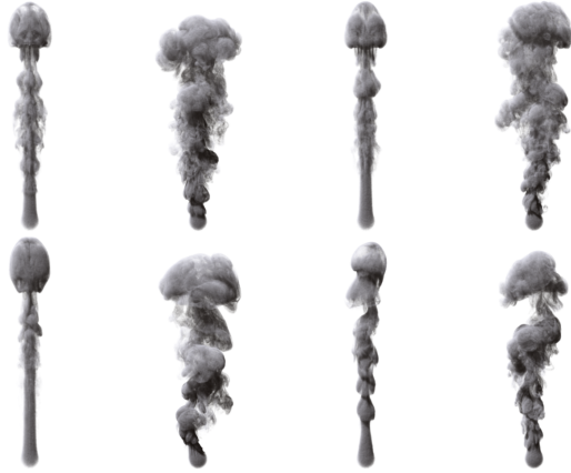
Figure 3.1: Rising smoke simulations with and without IVOCK (Integrated Vorticity of Convective Kinematics). From top left to bottom right, : Stable Fluids, Stable Fluids with IVOCK; BFECC, BFECC with IVOCK; MacCormack, MacCormack with IVOCK; FLIP, FLIP with IVOCK.
