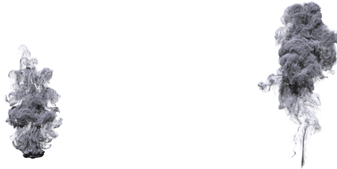
Figure 4.10: Without the far-field motion, direct summation using a cut-off kernel results in wrong animation. Left: simulation uses cut-off direct summation after 180 time steps. Right: simulation uses PPPM summation after 180 time steps.
