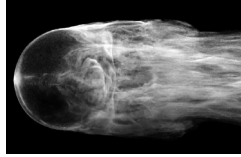
Figure 2.6: Impulsively started flow past a sphere at Re=15000 simulated using our solver
