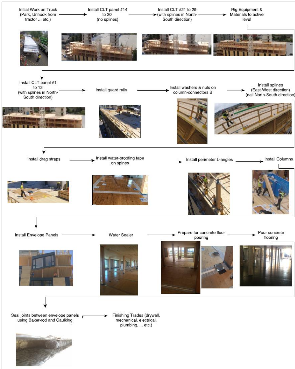
Figure 5: Sequence of structural elements
