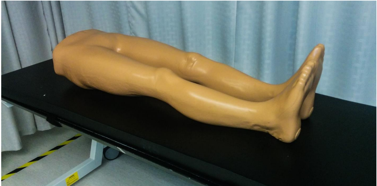
Figure 4: Manikin with radiodense bones used for AXIS
