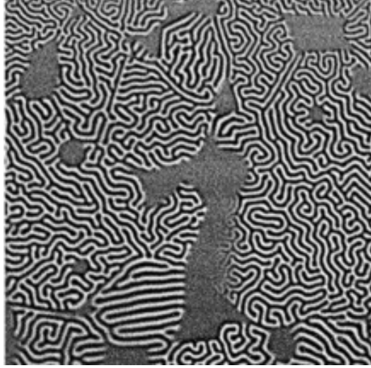
Figure 2.8: Scanning transmission X-ray microscopy image of 20 \mu\text{m} \times 20 \mu\text{m} Nd-Fe-B sintered magnet with thickness 50 – 150 nm. Maze-like domain patterns are clearly observed. This figure is adapted from Ref. [22].
