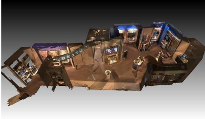
Figure 6.5: 3D as-built model generated via Tango which is then tested for dimensional accuracy.
