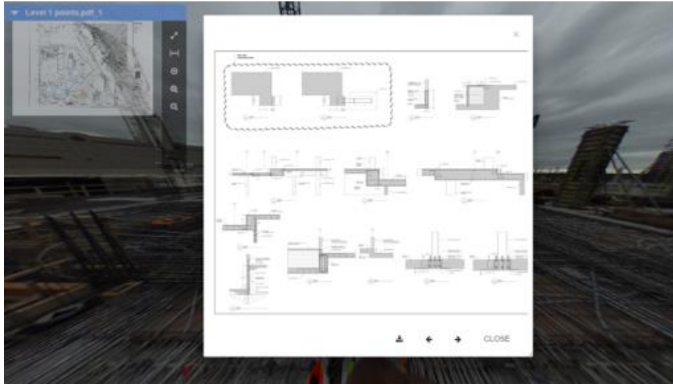
Figure 6.19: Sample image showcasing how the project team members were able to simultaneously access the relevant section plans at the necessary location.
