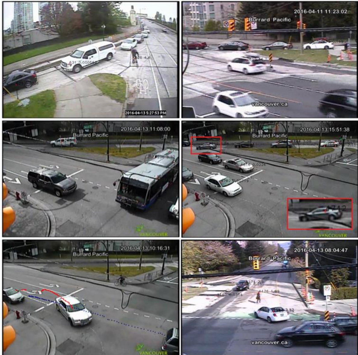
Figure 3-41: Examples of violations: not-yielding (top-left), cross blocking (top-right), stopping beyond the crossing traffic lines (mid-left), changing lanes over solid traffic paint lines (mid-right), using the wrong lane (bottom-left), and illegal right-turn (bottom-right).
