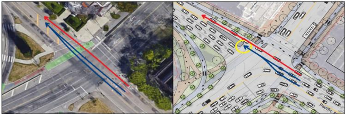
Figure 3-53: Lane-switching correction for the Pacific St. WB approach by the new traffic island.
