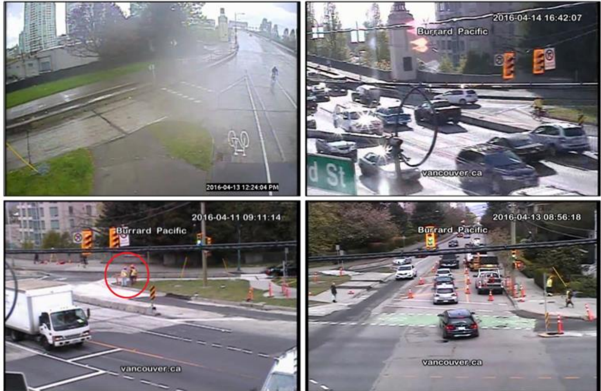
Figure 3-51: Challenges caused by bad weather (top-left), sun glare (top-right), traffic control personnel (bottom-left), and traffic control operations (bottom-right).
