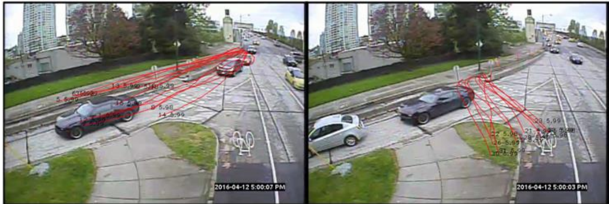
Figure 3-19: Sample prototypes for road user movements: vehicles (left) and cyclists (right) (S2 example).
