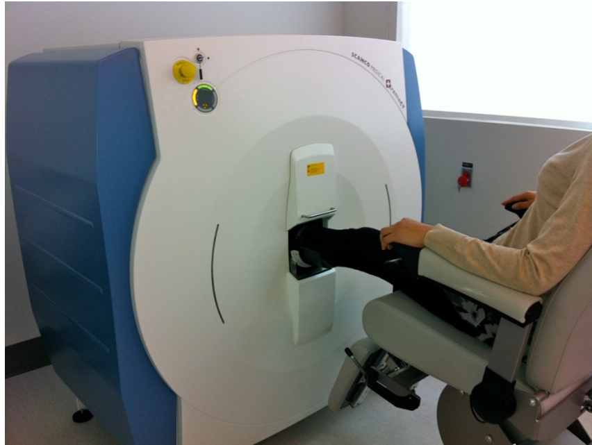
Figure 1.14. Image of high-resolution peripheral quantitative computed tomography (HR-pQCT) XtremeCT system (Scanco Medical) and leg positioning for tibia scan.
