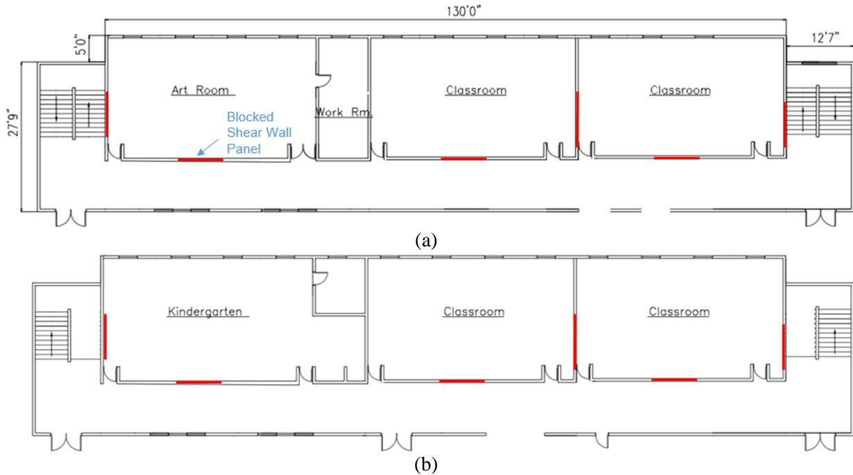
**Figure 47: Blocked shear wall retrofit solution for Institutional Archetype for (a) Floor 1, (b) Floor 2**
