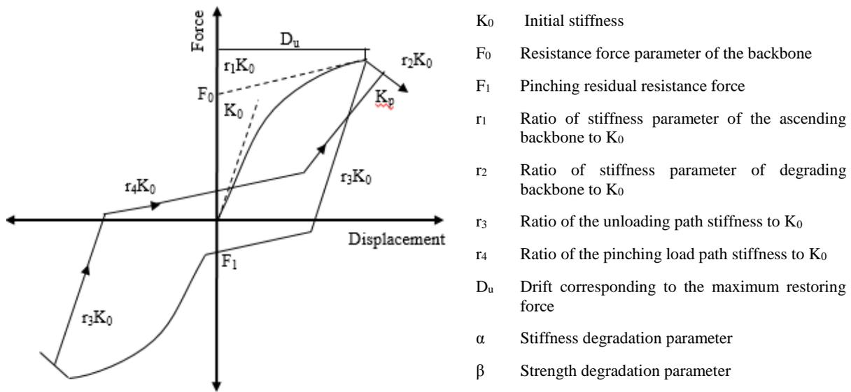
**Figure 3: Loading paths and parameters of MSTEW material model**
