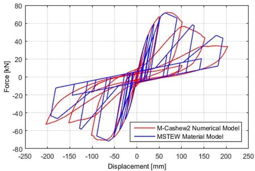
**Figure G.9: MSTEW model fit to hysteretic loops for pretest Classroom wall model**
