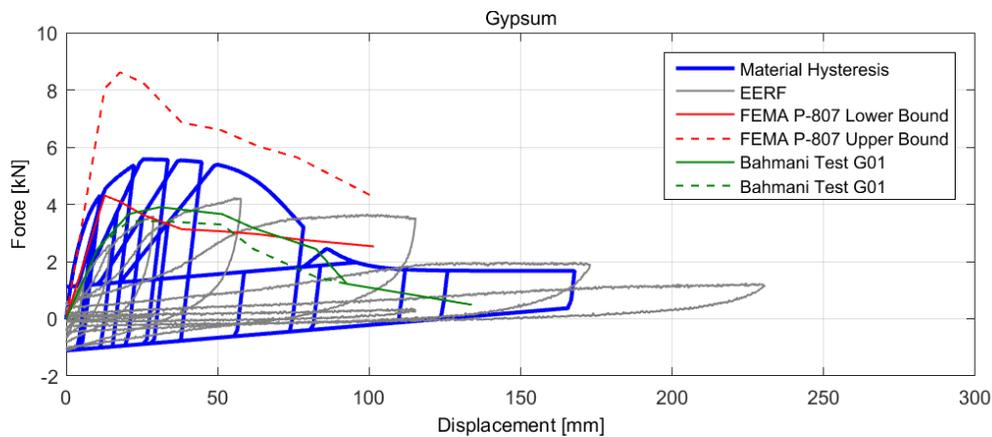
**Figure 29: Gypsum Material Model compared to experimental data (8ft wall segment)**
