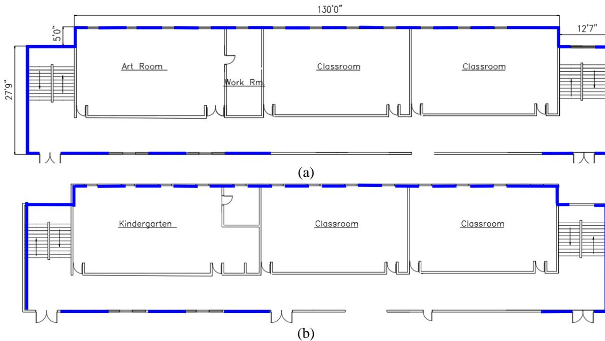
Figure 50: Proposed stucco retrofit solution for Institutional Archetype for (a) Floor 1, (b) Floor 2
