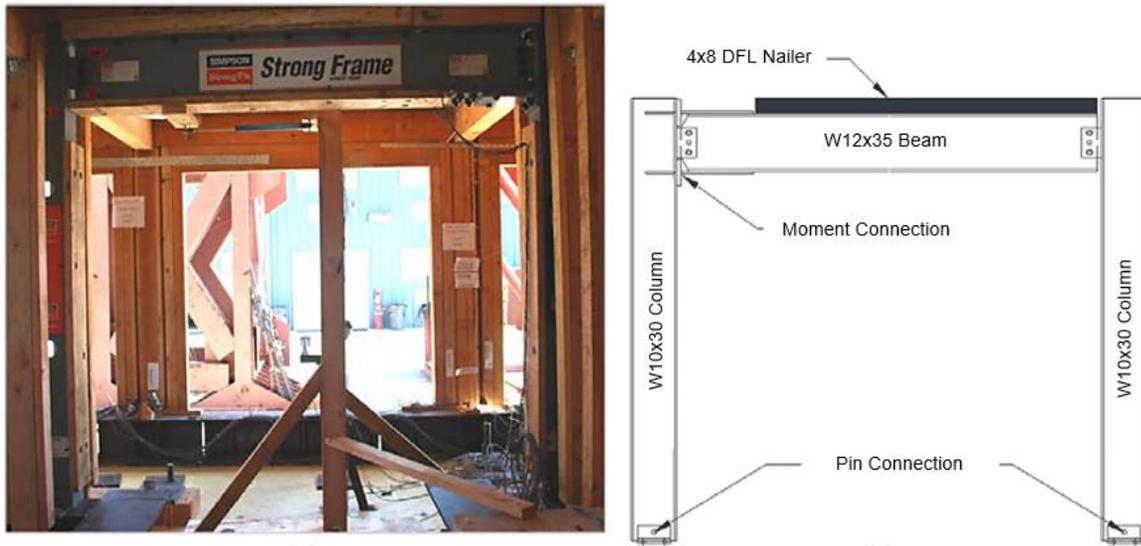
Figure 55: Strong Frame SMF a) Installed in first “soft” storey retrofit full scale test b) elevation of details (Bahmani, et al., 2014)
