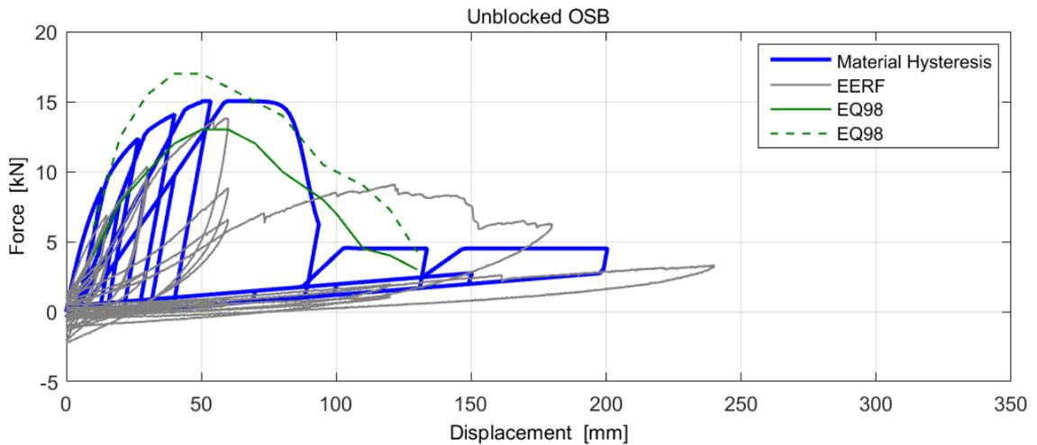
**Figure 12: Unblocked shear wall model compared to experimental data**
