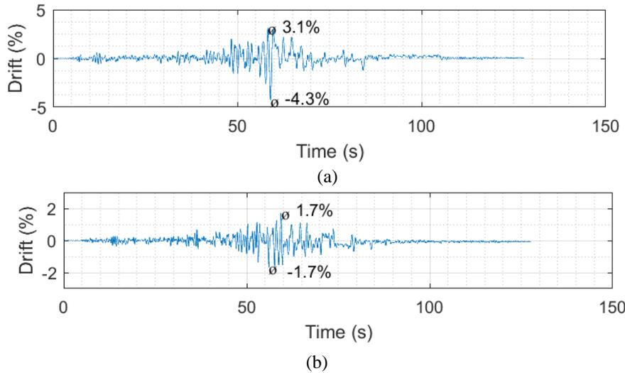
**Figure 30: Prediction of the time history to the pretest acceleration output of the shake table for: (a) the segmented method Timber3D model, (b) the recommended FEMA P-807 Timber3D model**
