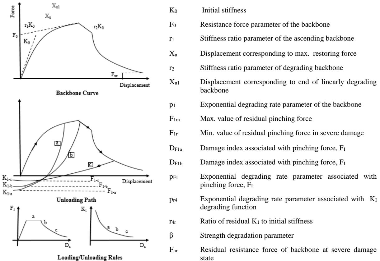
**Figure 4: Loading paths/parameters for EPHM 16 parameter material hysteresis by Pei and van de Lindt (2010)**
