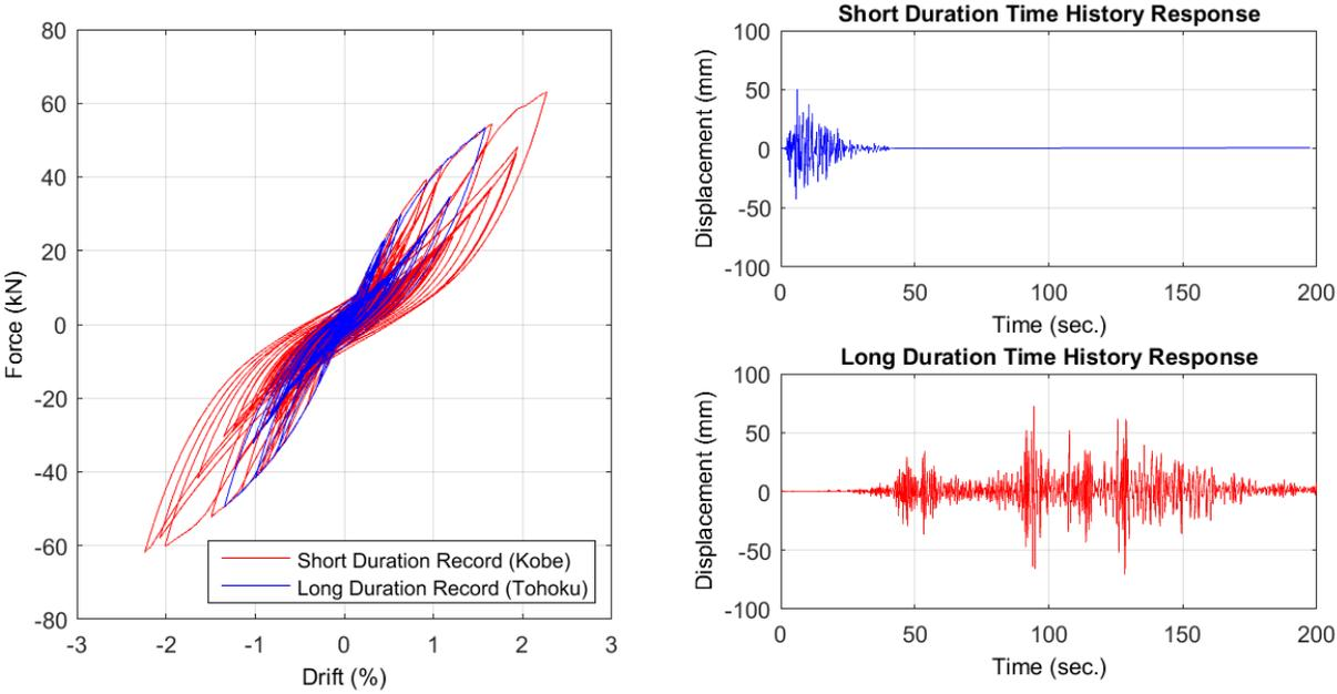
**Figure 38: Comparison of numerical analysis results for Kobe (Short) and Tohoku (Long) spectrally equivalent ground motions (a) hysteresis, (b) displacement time-history**
