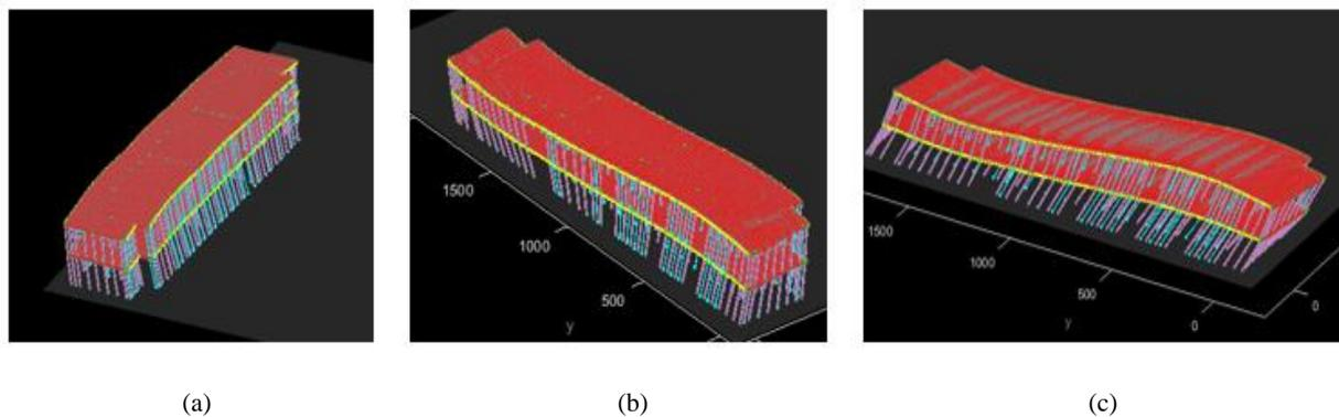
**Figure 43: Modes of Vibration: (a) north-south, (b) torsional, (c) east-west**
