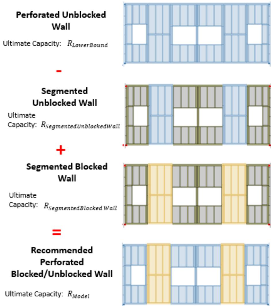
Figure G.11: Recommended Perforated Wall Ultimate Capacity
