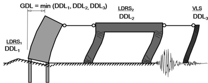
**Figure D.3: Governing drift limit for system for the 'Toolbox Method'**
