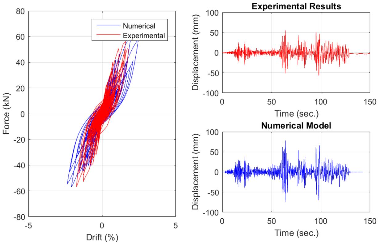
**Figure G.7: Run 1 comparison of numerical and experimental hysteretic and time-history response**
