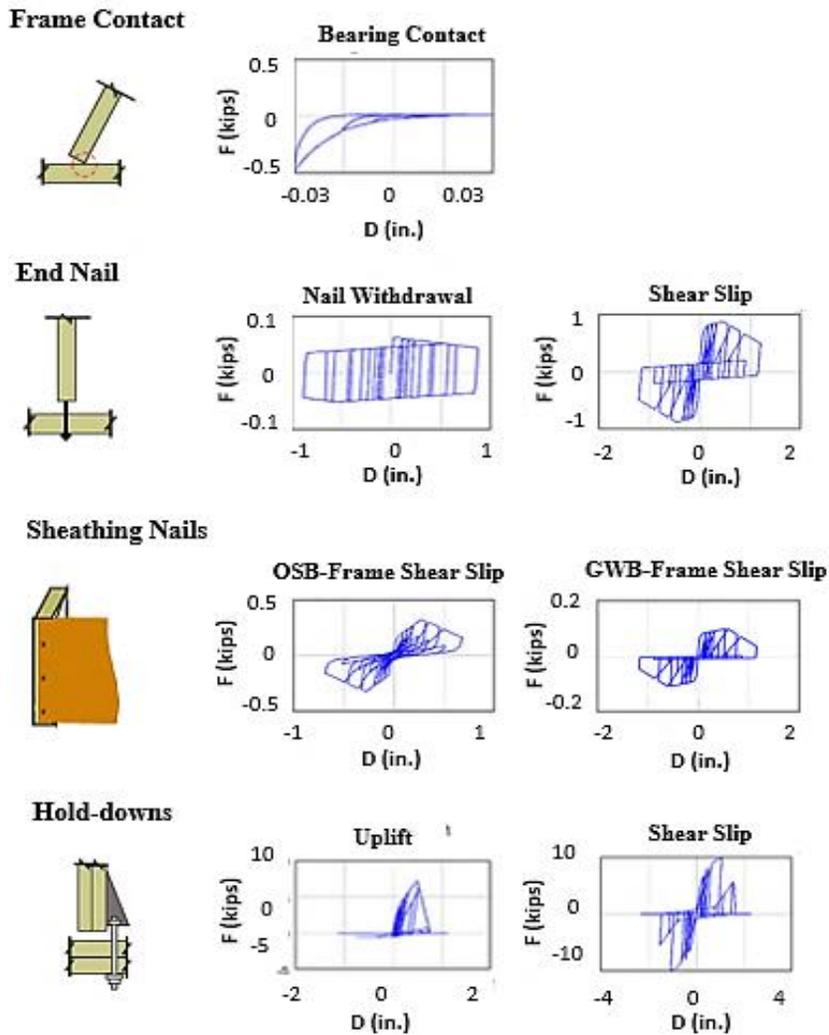
Figure G.4: Hysteretic models for (a) frame contact, (b) end nails, (c) sheathing nails, and (d) PHD5 Hold-downs, (van de Lindt J. W., Pei, C., & Hassansadeh, 2012b)
