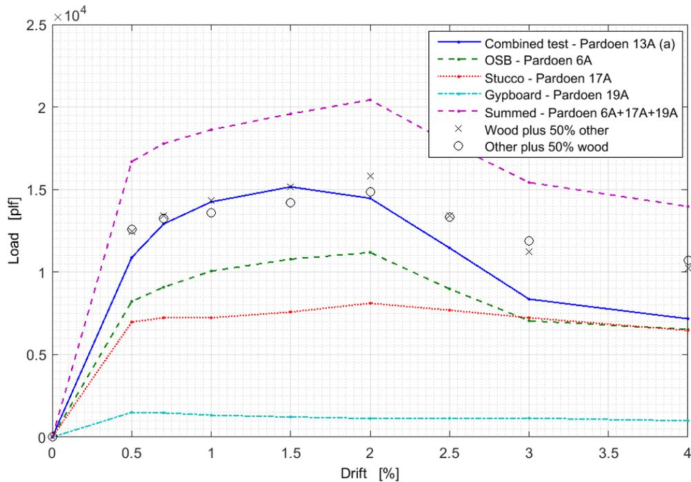
**Figure D.1: Separate and combined wall tests for OSB, Stucco and Gypsum Boards compared to 100%/50% rule proposed in the FEMA P-807 Guidelines (FEMA, 2012)**
