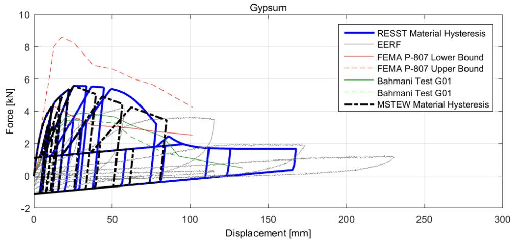
**Figure 45: Gypsum Material Model compared to experimental data (8ft. wall)**
