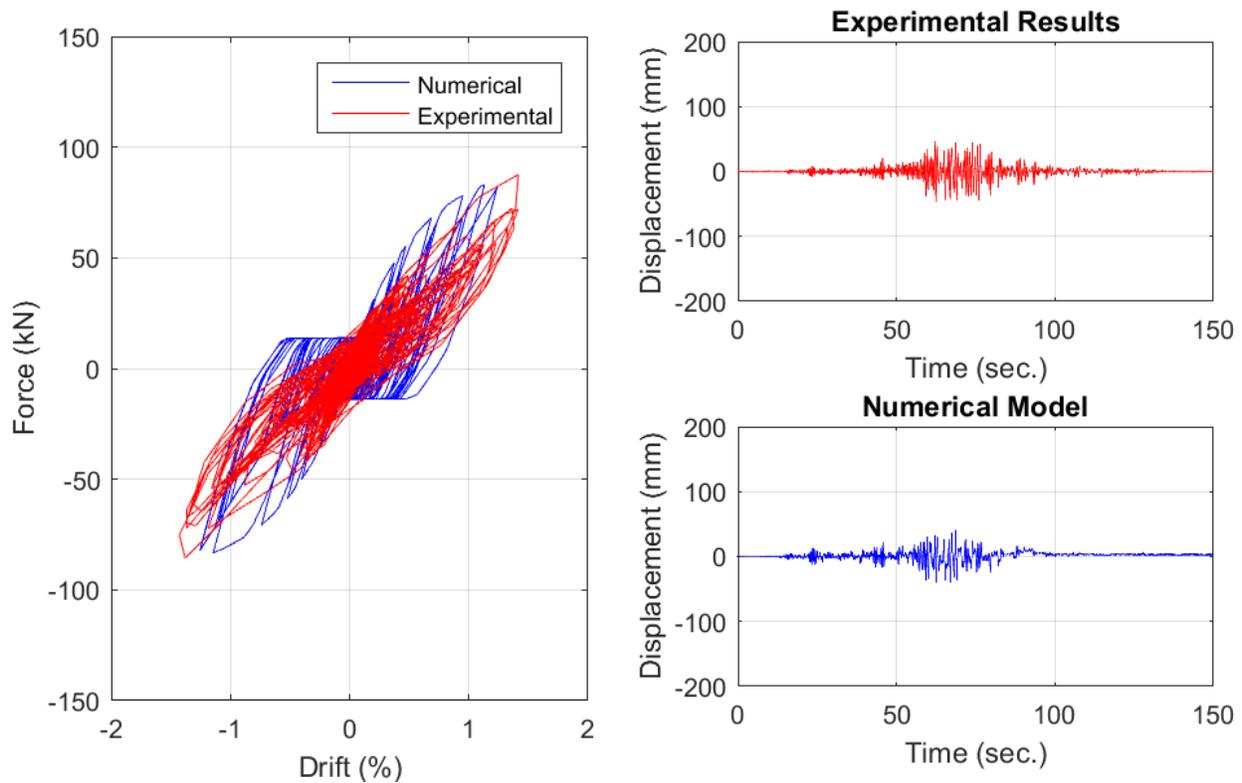
Figure 33: Global Numerical Model and Experimental (a) hysteresis (b) displacement time history for Run 1
