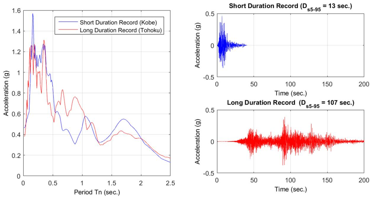
**Figure 36: Kobe and Tohoku spectrally equivalent records (a) response spectra (5% damping) and (b) time history of short and long duration records**
