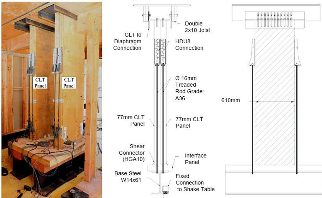
**Figure 52: Cross Laminated Timber (CLT) rocking walls for retrofit solution: a) Installed in first storey for full-scale testing and b) elevation and design details (Bahmani, et al., 2014).**
