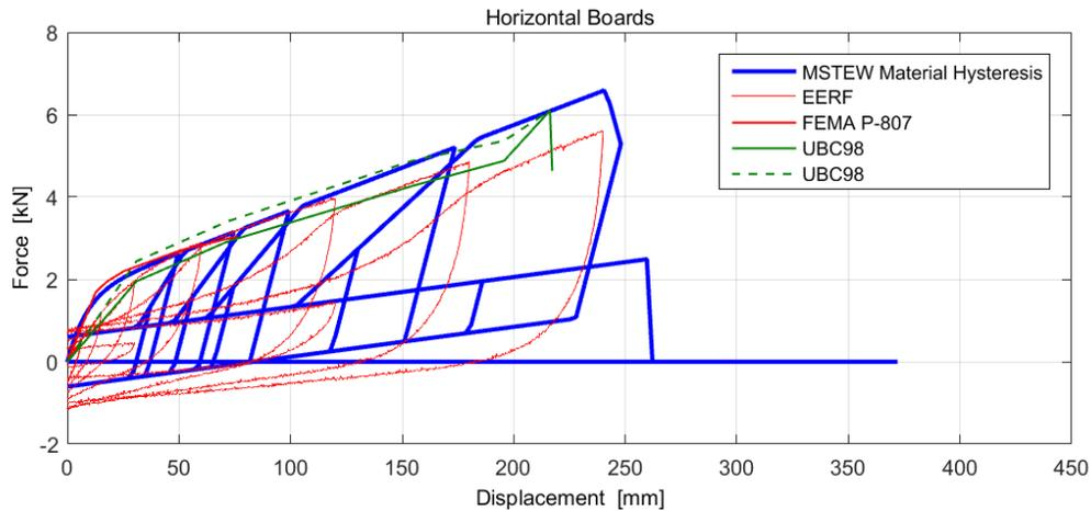
**Figure 46: Shiplap Material Model compared to experimental data (8ft. wall)**
