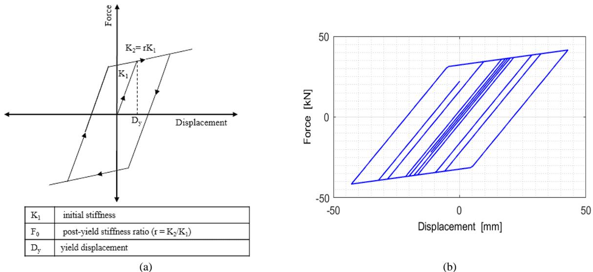
**Figure 54: (a) Details for Bilinear material model (b) Bilinear material model for SMF for Col.:W10x30 Beam:W12x35SMF**
