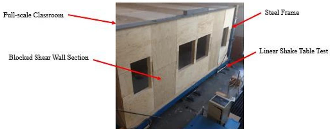
Figure G.1: Test Structure for Second Testing Configuration
