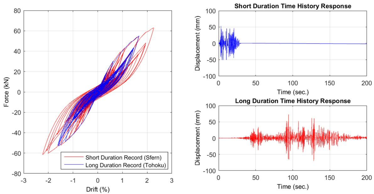
**Figure 39: Comparison of numerical analysis results for Sfern (Short) and Tohoku (Long) spectrally equivalent ground motions (a) hysteresis, (b) displacement time-history**
