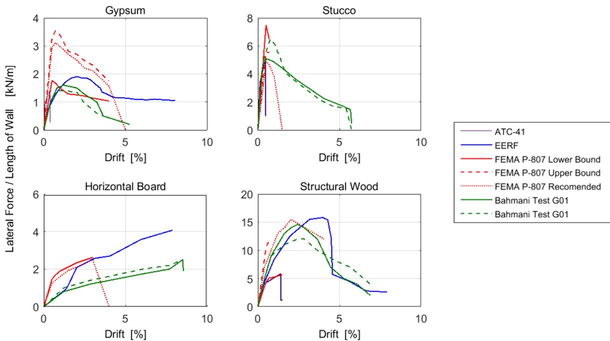
**Figure D.2: Comparison of backbones from the experimental tests by Bahmani and EERF and FEMA P-807 and ATC-41 data for (i) gypsum, (ii) stucco, (iii) horizontal board and (iv) structural wood**
