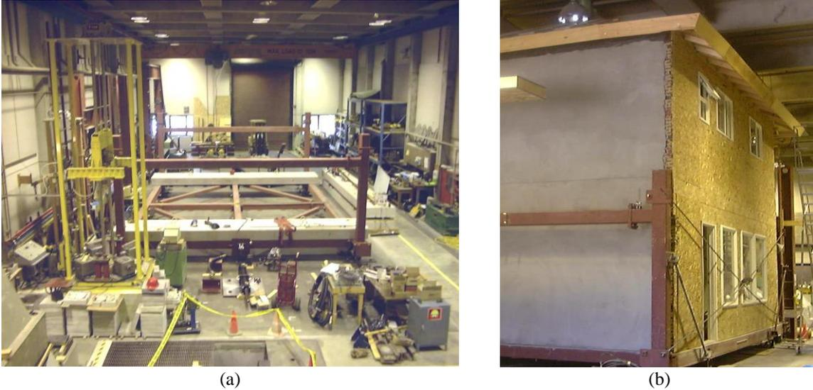
**Figure 8: Photograph of (a) Linear shake table, (b) Type 2 full-scale house**
