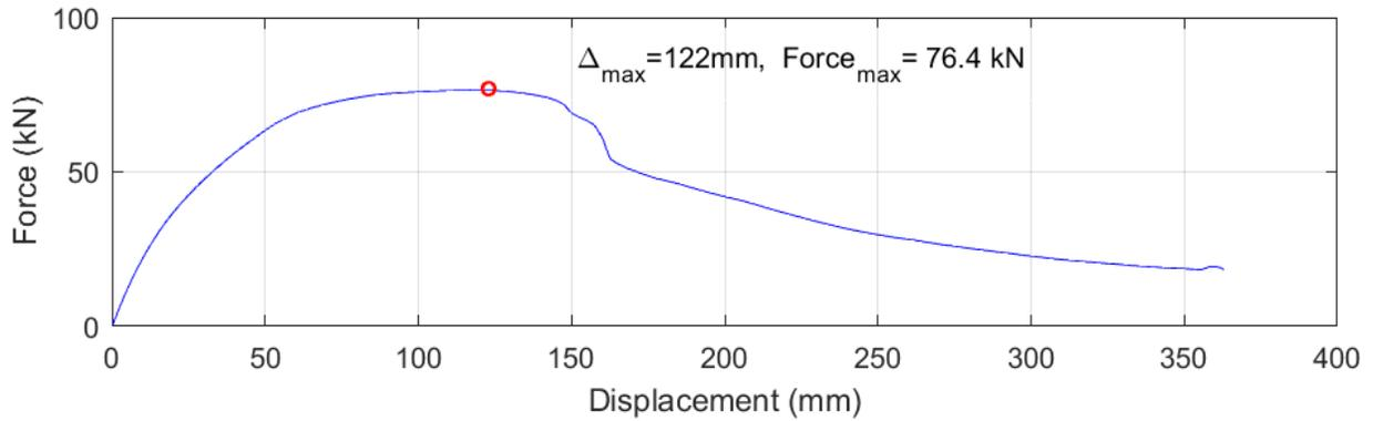
**Figure 24: Monotonic response of classroom shear wall numerical model**
