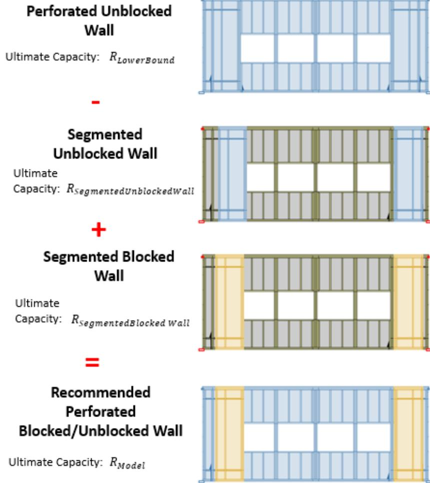
Figure 28: Recommended Perforated Wall Ultimate Capacity
