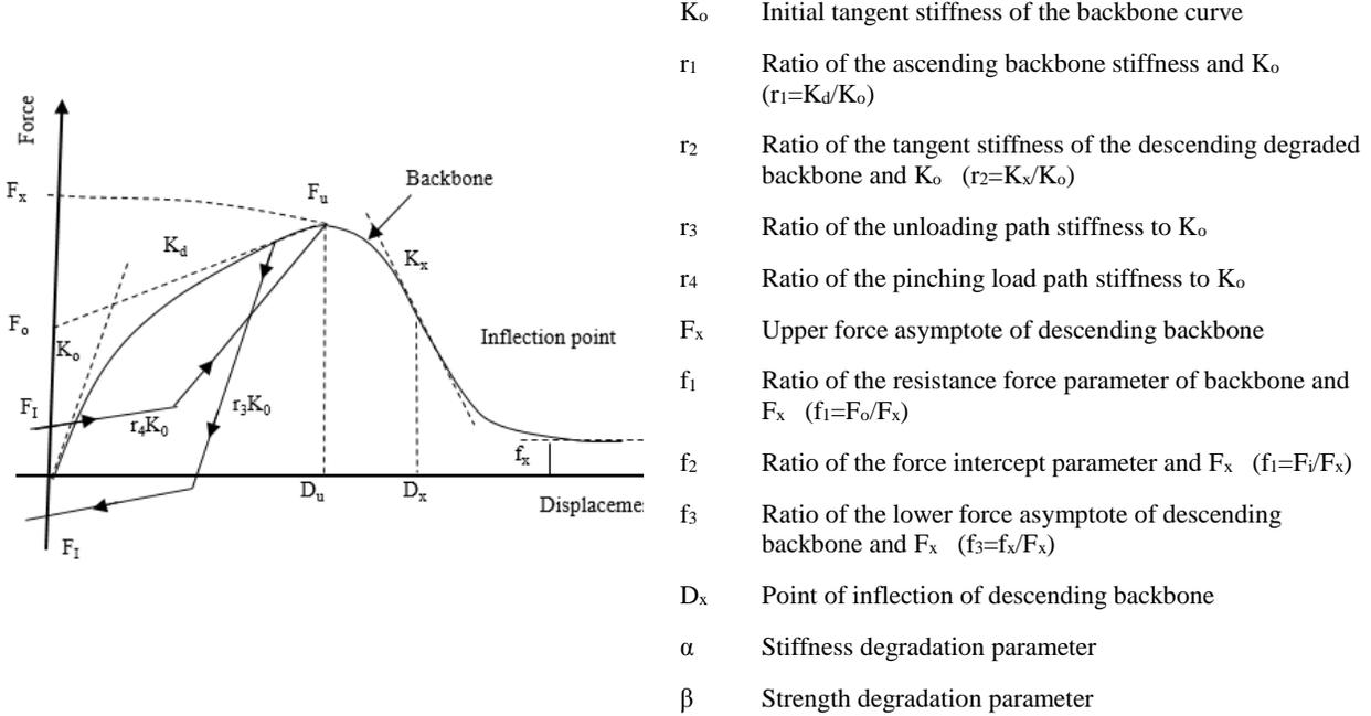
Figure 6: Loading paths and parameters of RESST material hysteresis model by Pang et al. (2007)
