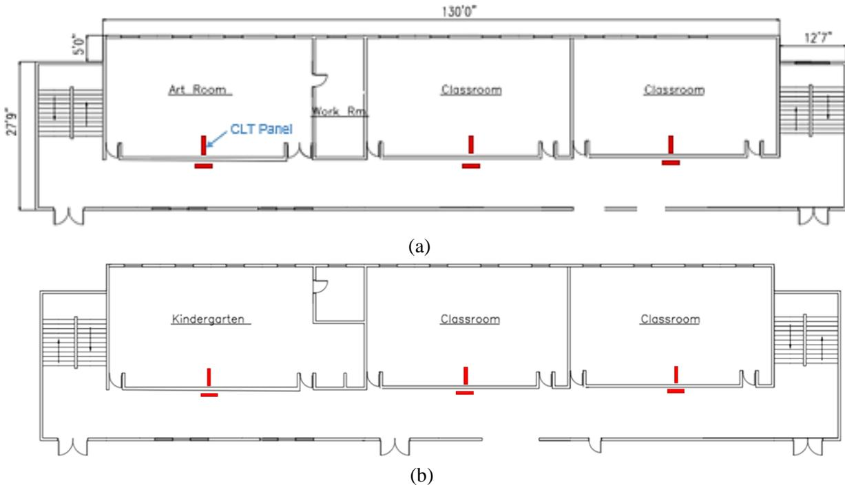
**Figure 53: Proposed CLT retrofit solution for Institutional Archetype for (a) Floor 1, (b) Floor 2**
