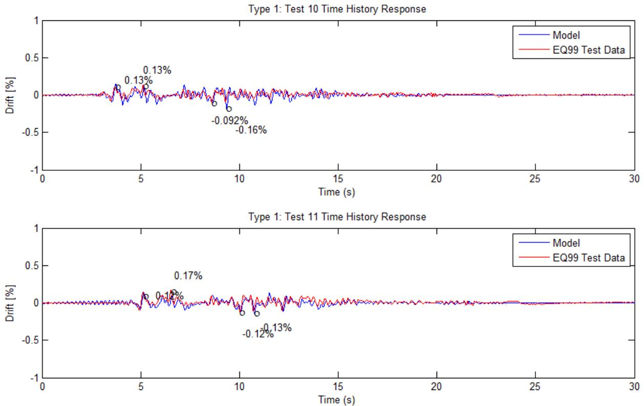
**Figure 15: Comparison of experimental and numerical results for Prototype 1 (Stucco, Blocked OSB, hold-downs)**
