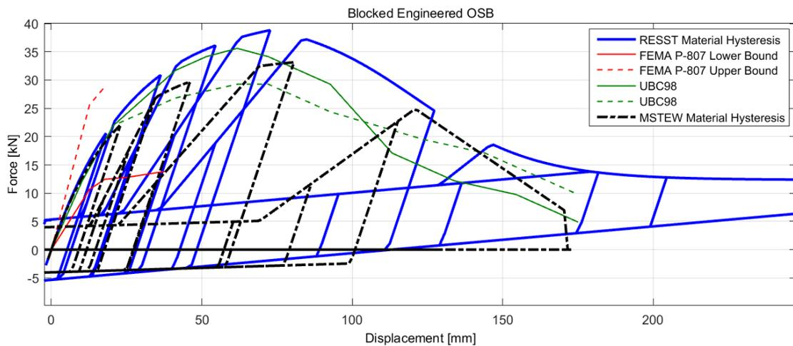
**Figure 48: Blocked Engineered shear wall material model compared to experimental data (8ft. wall)**
