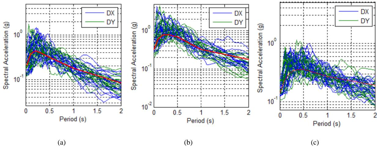
**Figure 61: Vancouver, B.C. 2% in 50 years' spectra for (a) crustal, (b) subcrustal, (c) subduction earthquakes**
