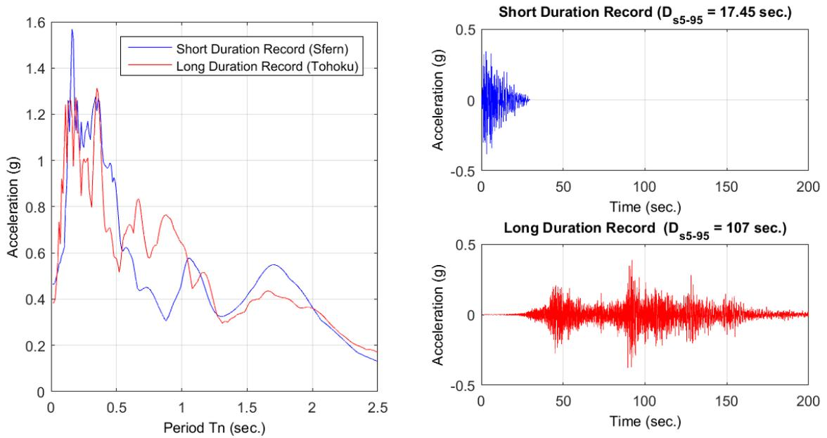
**Figure 37: Sfern and Tohoku spectrally equivalent records (a) response spectra (5% damping) and (b) time history of short and long duration records**
