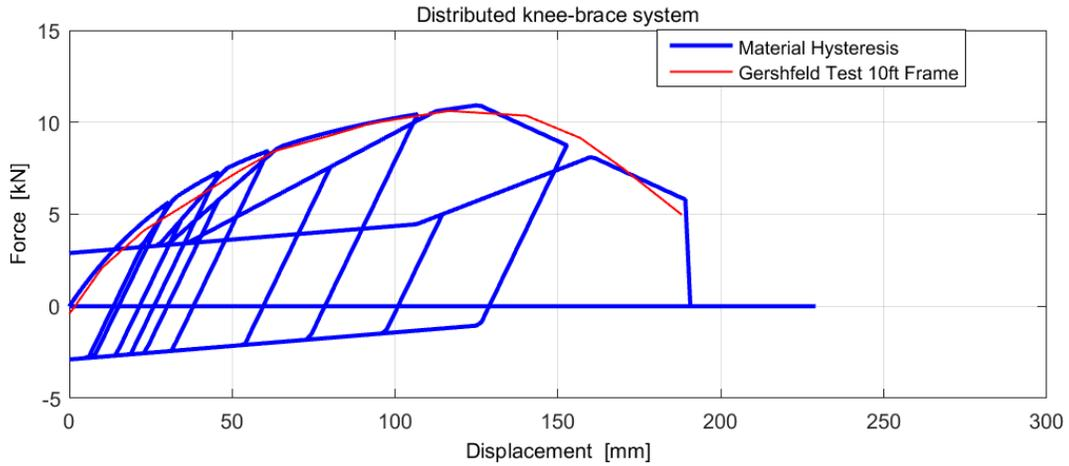
**Figure 58: Experimental and numerical hysteresis for distributed knee system for 10ft. four-frame assembly**
