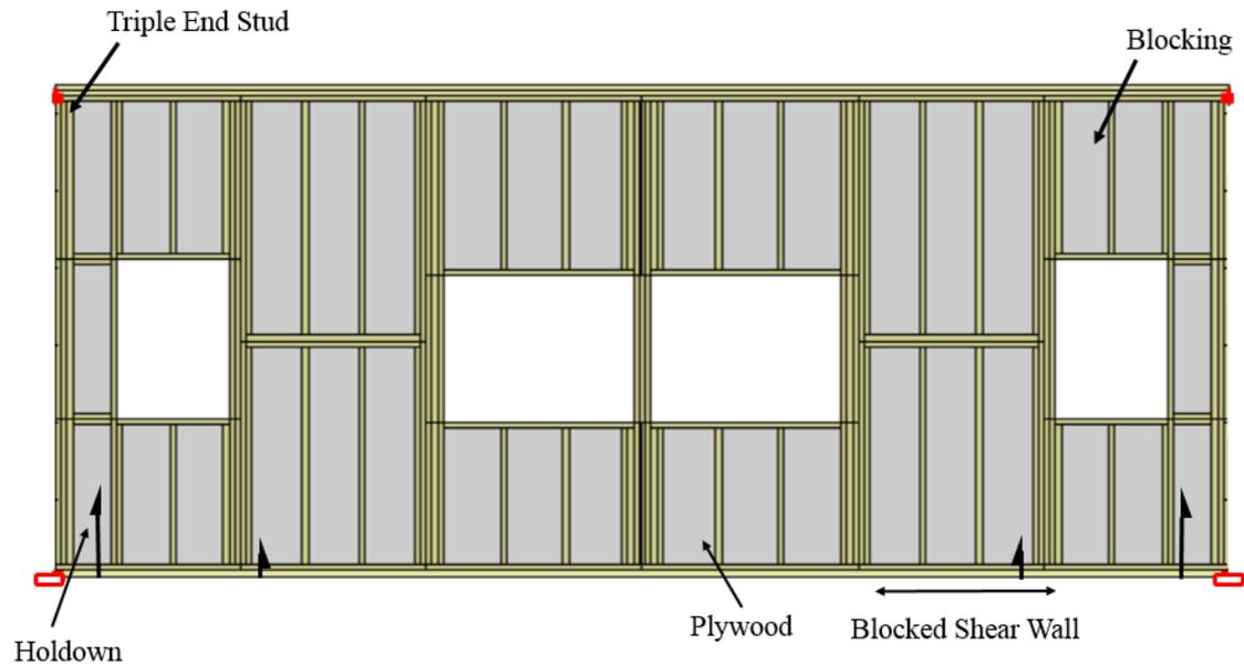
**Figure G.2: M-CASHEW2 Model of Classroom North and South Elevation for Second Testing Configuration Numerical Model**
