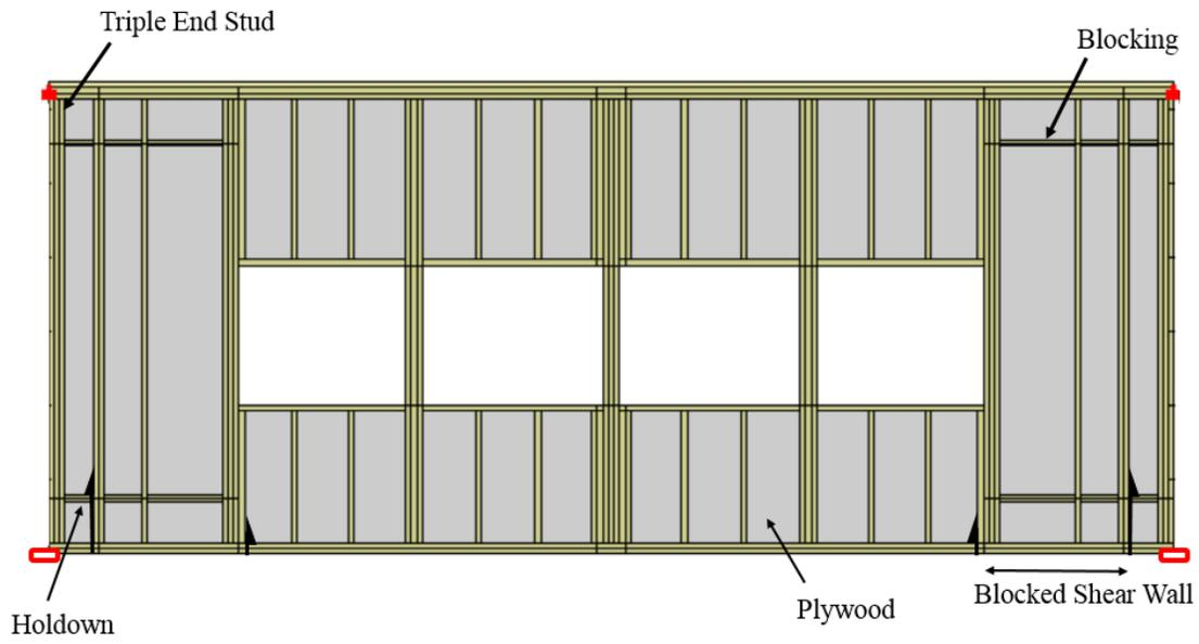
**Figure 20: M-CASHEW2 Model of Classroom North and South Elevation**
