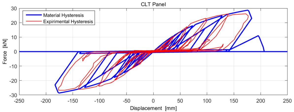
**Figure 51: Experimental and Numerical Hysteresis for single CLT panel wall**
