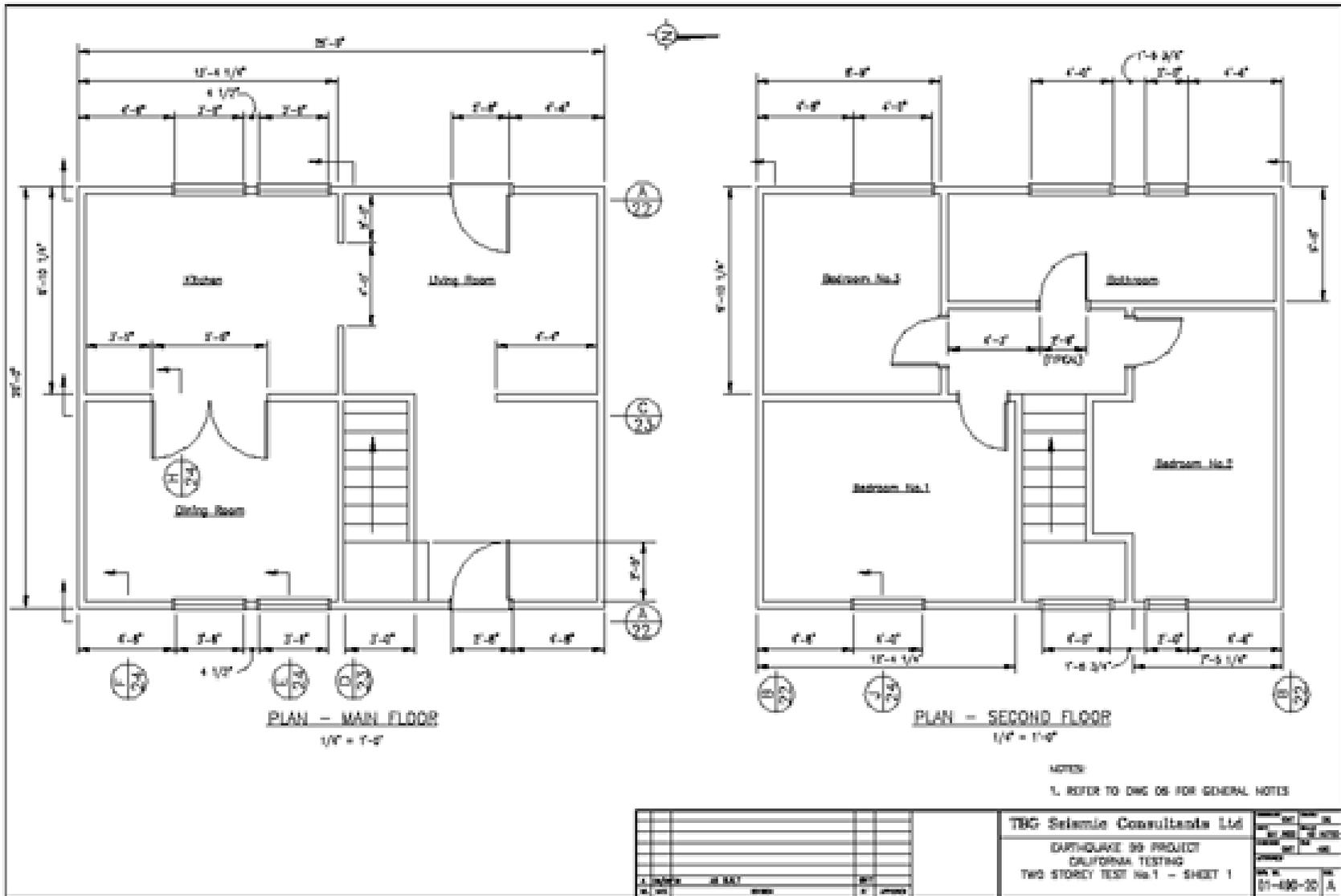
Fig. B.2: Two-storey woodframe house plan view
