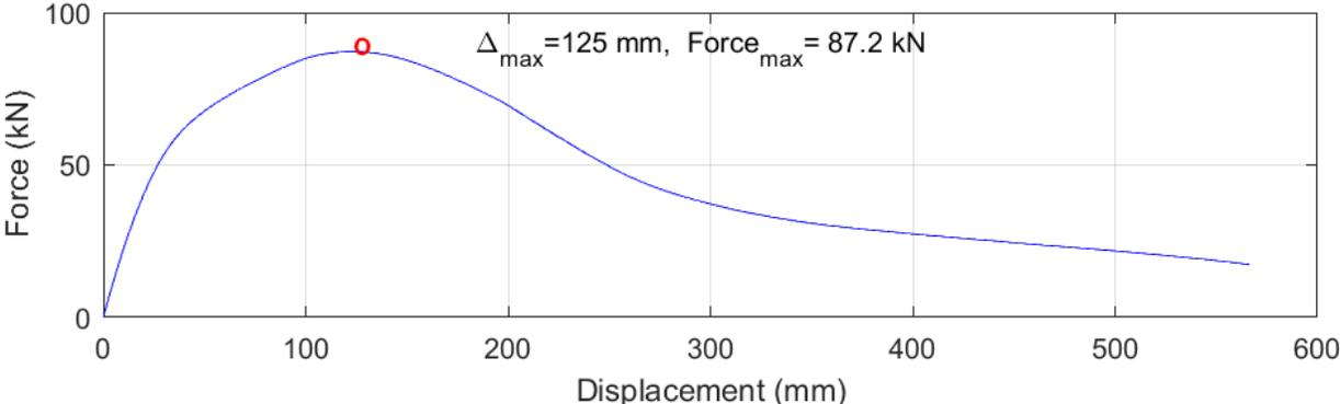
Figure G.5: Monotonic response of classroom shear wall numerical model
