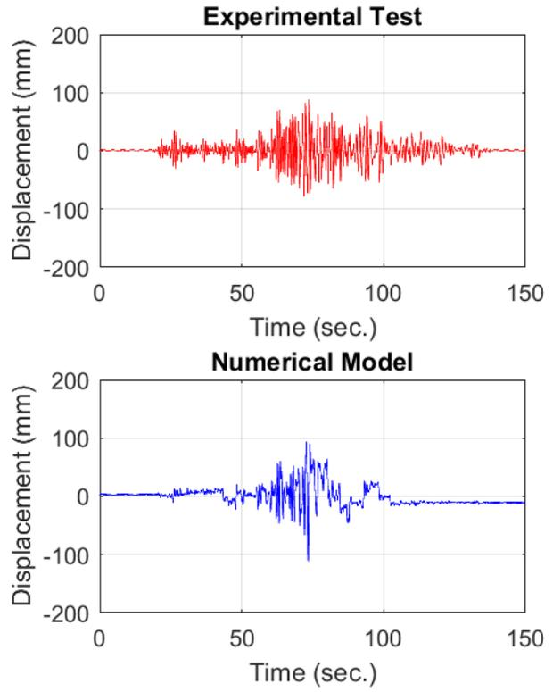
Figure 34: Global Numerical Model and Experimental (a) hysteresis (b) displacement time history for Run 2
