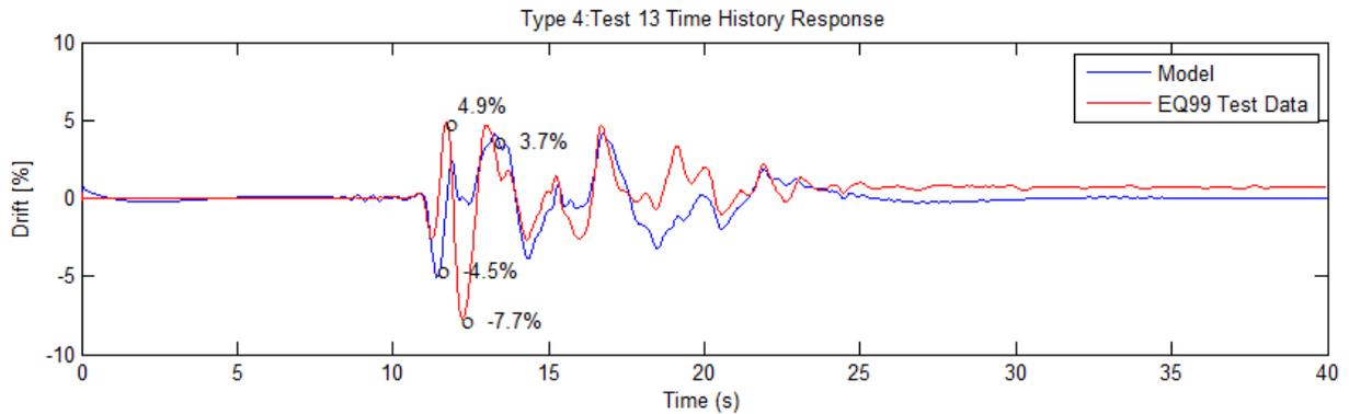
**Figure 18: Comparison of experimental and numerical results for Prototype 4 (Horizontal Boards)**
