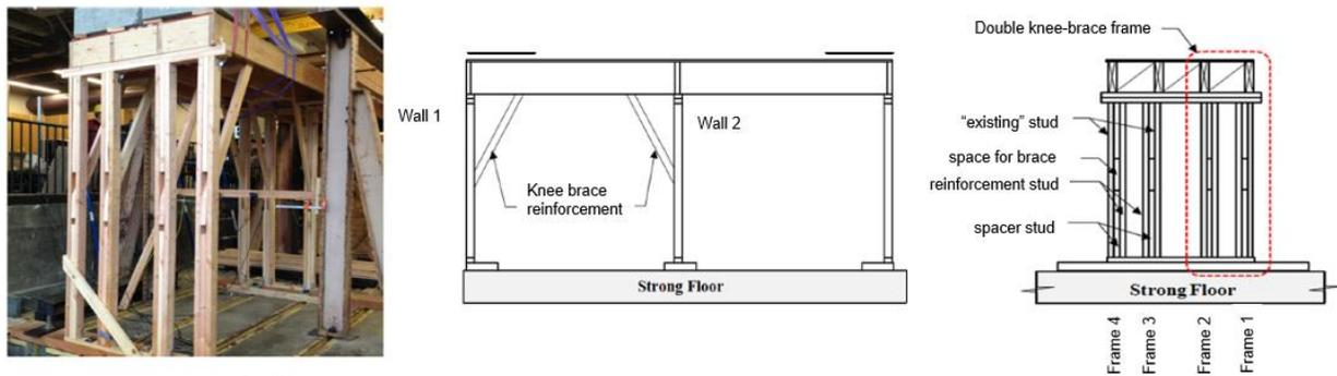
Figure 57: DKB System: a) Testing of system b) elevation view of details (Gershfeld M. , et al., 2014)
