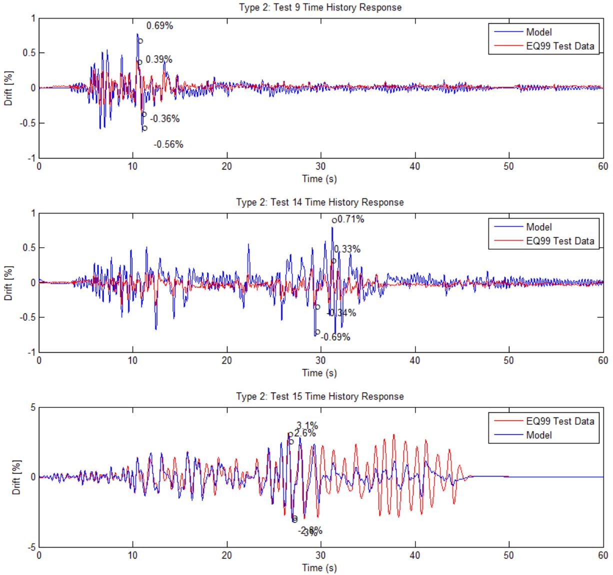
**Figure 16: Comparison of experimental and numerical results for Prototype 2 (Blocked OSB, hold-downs)**
