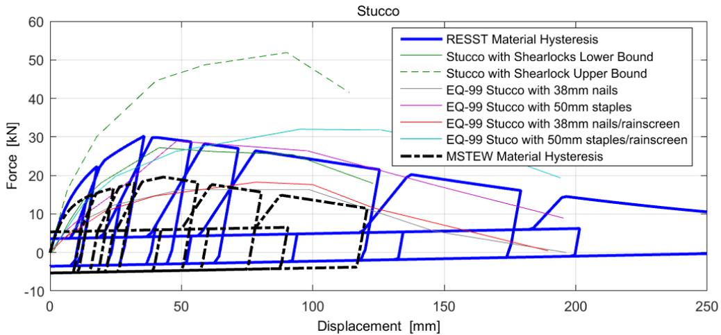
Figure 49: New stucco construction shear wall material model compared to experimental data (8ft. wall)
