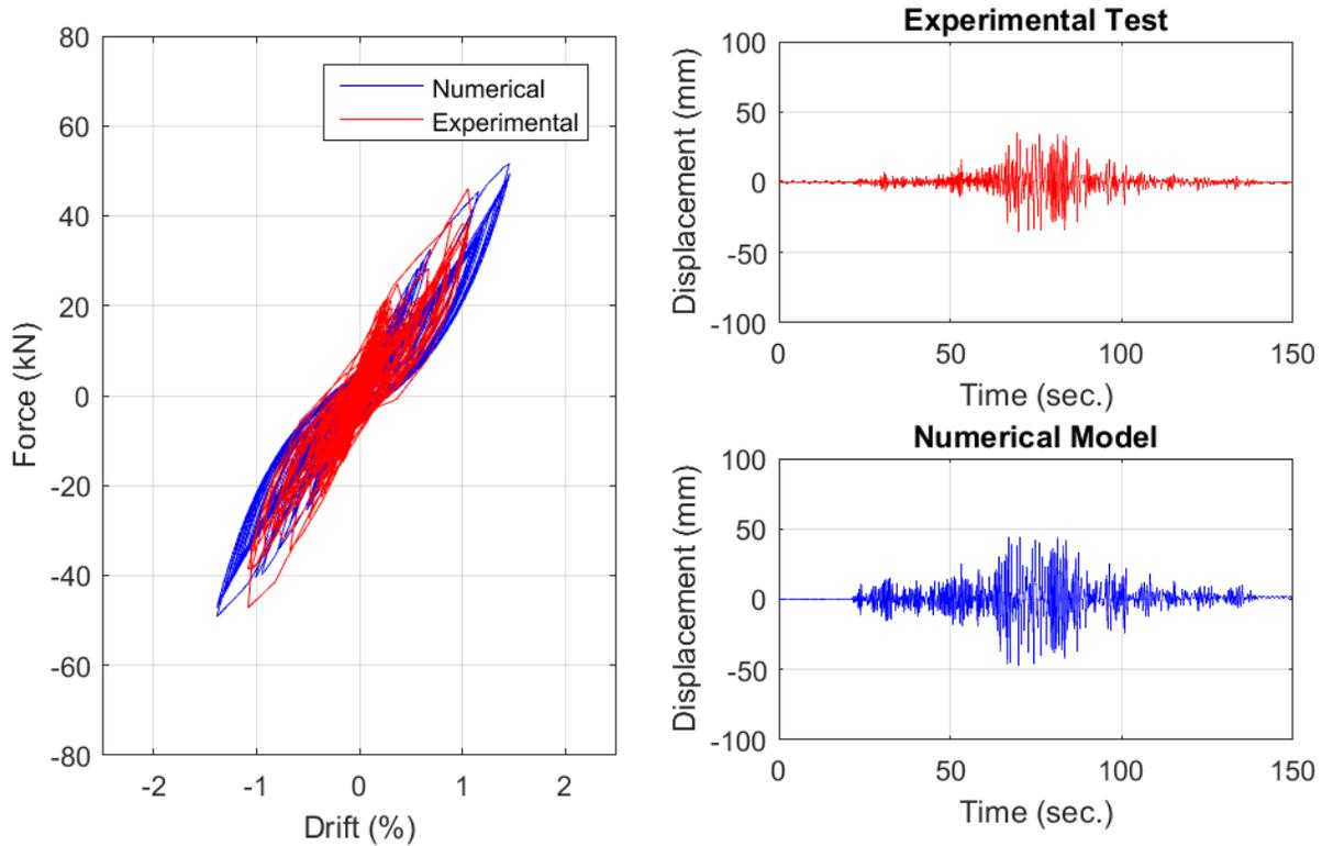
Figure 31: Detailed Numerical Model and Experimental (a) hysteresis (b) relative displacement time history for Run 1
