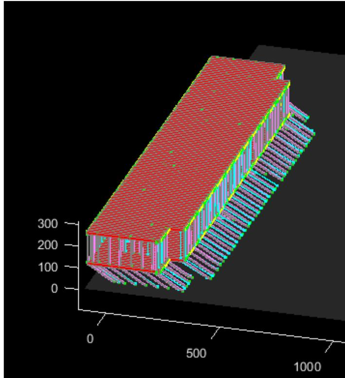
Figure 64: Deformed shape at incipient of collapse of school block
