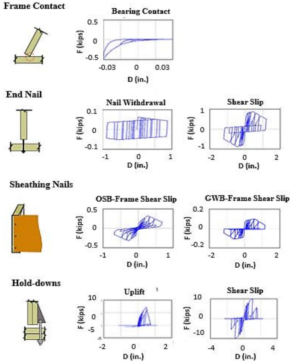
**Figure 23: Hysteretic models for (a) frame contact, (b) end nails, (c) sheathing nails, and (d) PHD5 Hold-downs, (van de Lindt J. W., Pei, C., & Hassansadeh, 2012b)**
