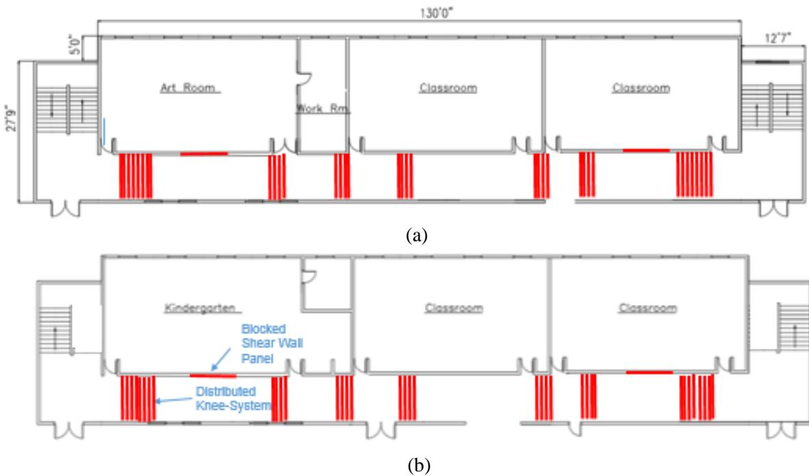
**Figure 59: Proposed distributed knee system and blocked shear wall panel retrofit solution for Institutional Archetype for (a) Floor 1, (b) Floor 2**
