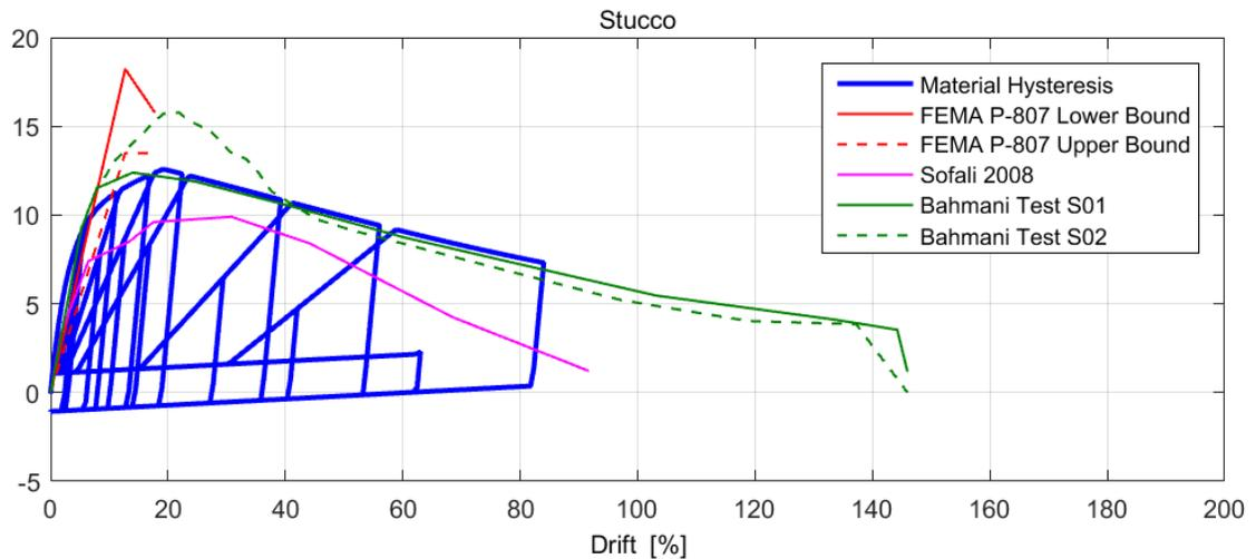
**Figure 14: New stucco construction shear wall material model compared to experimental data (8ft. wall)**
