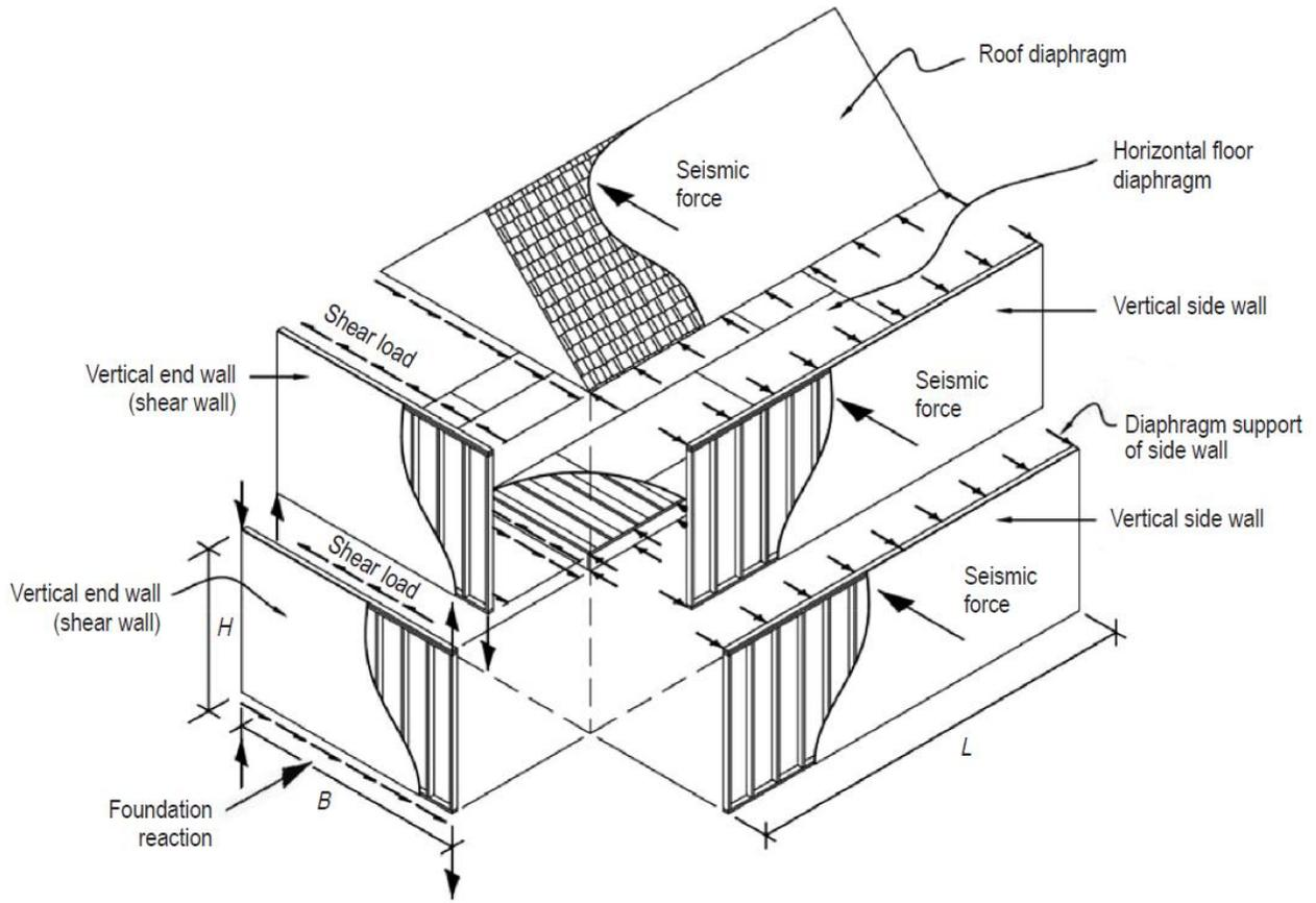
Figure 1: Light-frame wood building with load path illustrated (Toothman, 2003)
