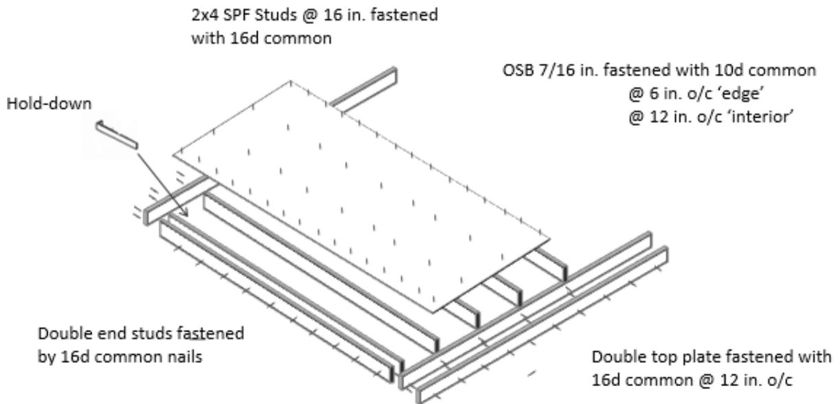
Figure 2: Typical Shear wall construction (Heine, 1997)
