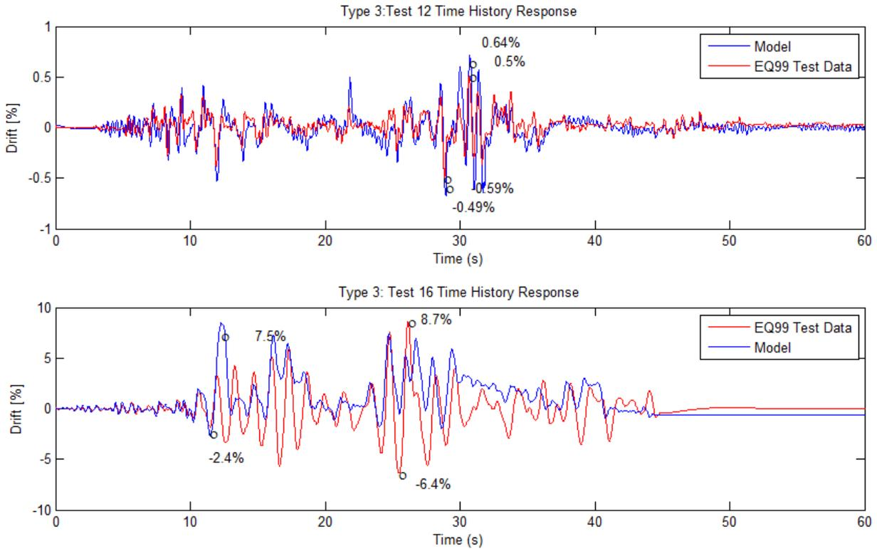
**Figure 17: Comparison of experimental and numerical results for Prototype 3 (Unblocked OSB)**
