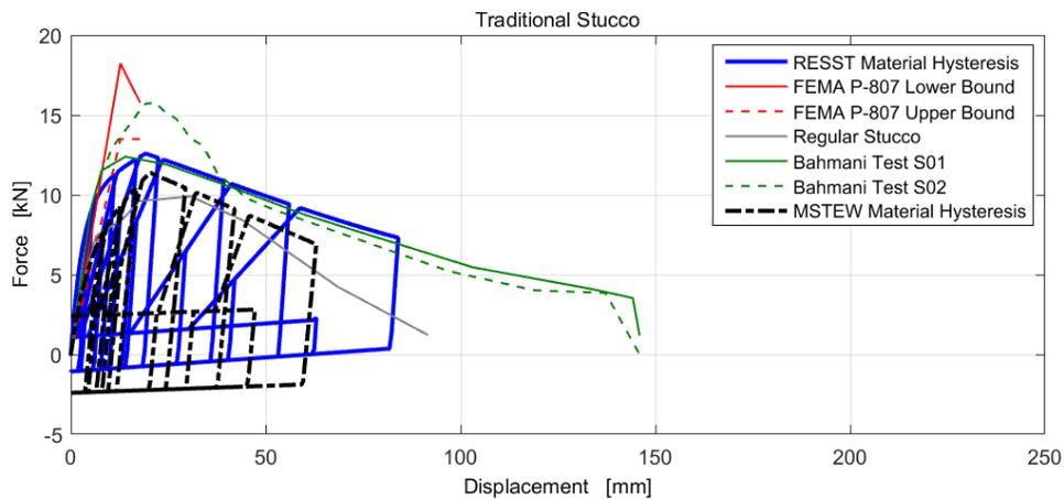
**Figure 44: Stucco Material Model compared to experimental data (8ft. wall)**
