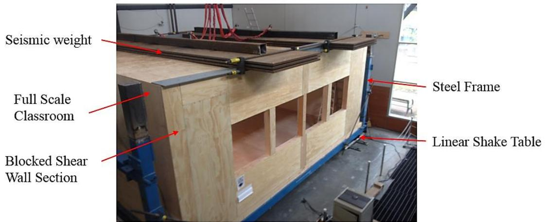
**Figure 21: Photograph of test setup prior to testing**
