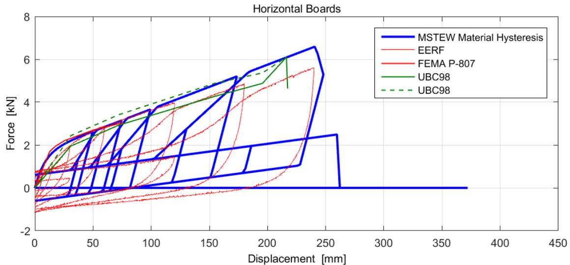
**Figure 13: Horizontal Board Material Model compared to experimental data**
