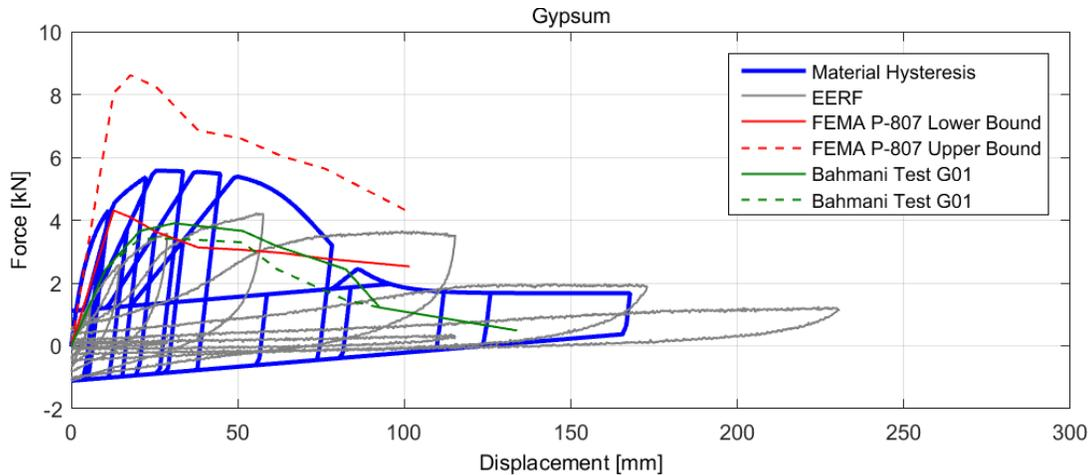
**Figure 10: Gypsum Material Model compared to experimental data**
