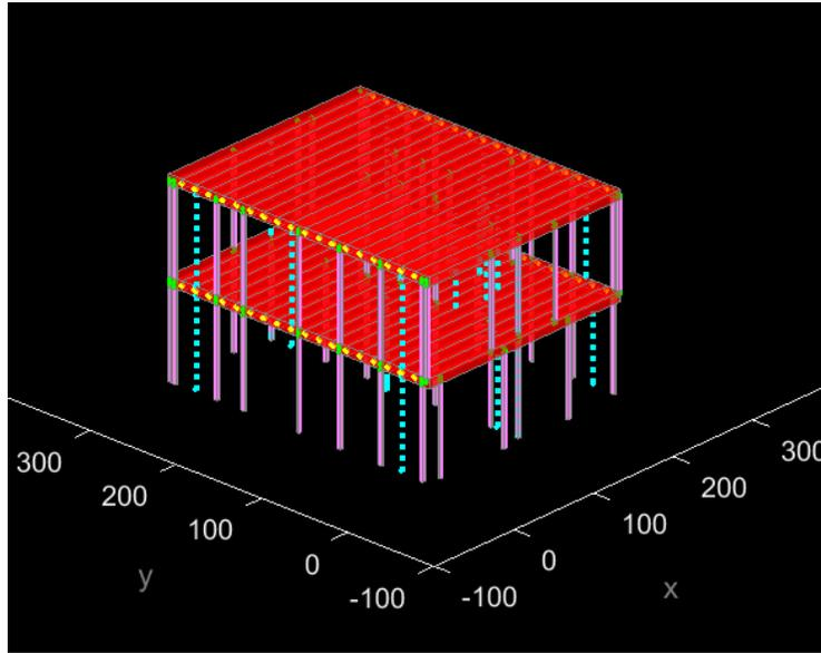
Figure 9: Modelling light-frame house with Timber 3D
