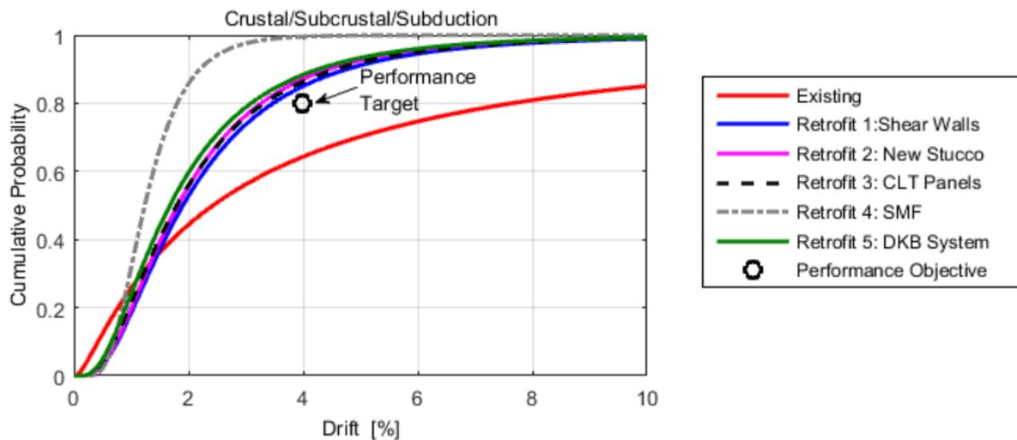
**Figure 63: Comparison of non-exceedance probability distributions from NLTHA of Existing Building and Retrofit Options**
