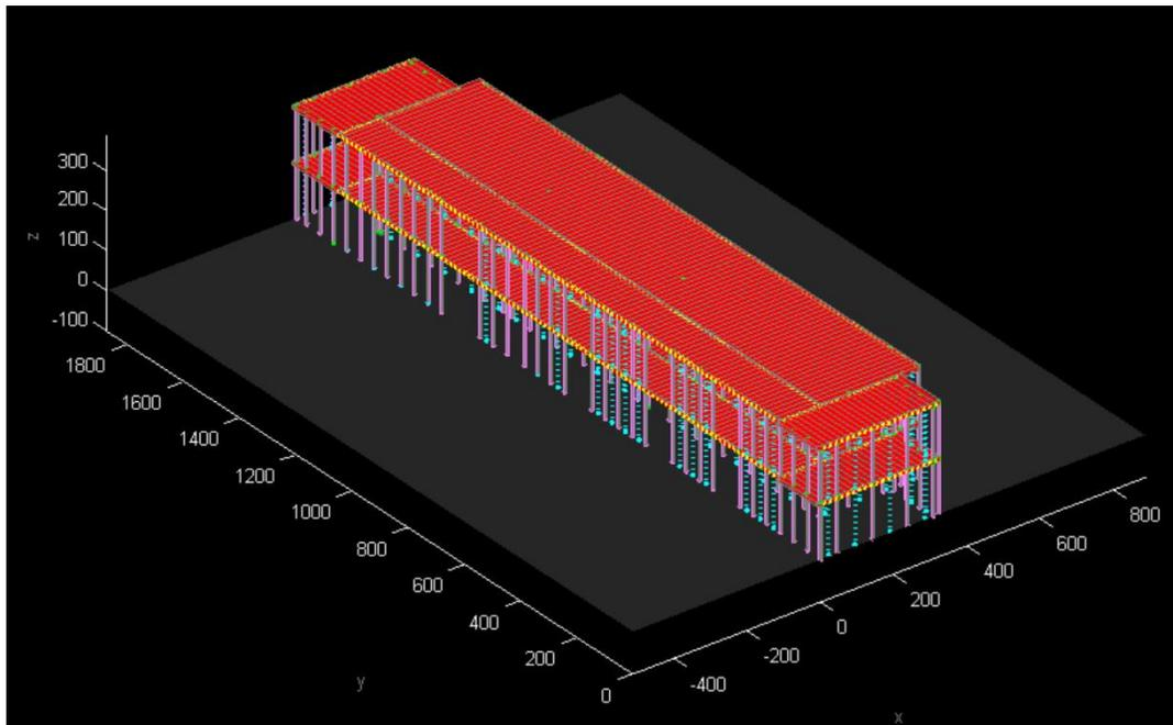
Figure 42: Modelling light-frame school block with Timber 3D
