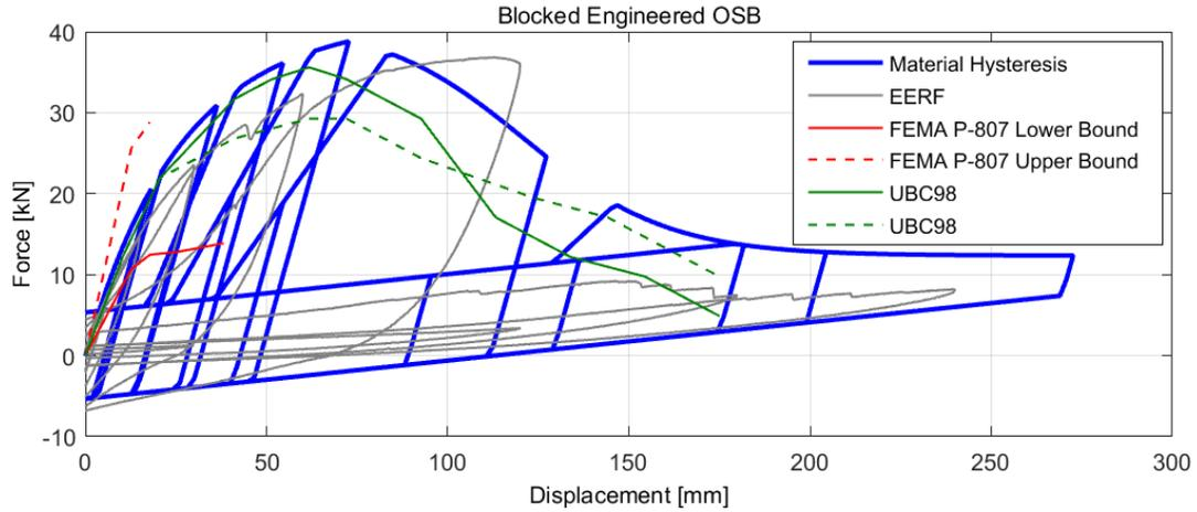
**Figure 11: Blocked Engineered Wood Shear Wall Material Model compared to experimental data**
