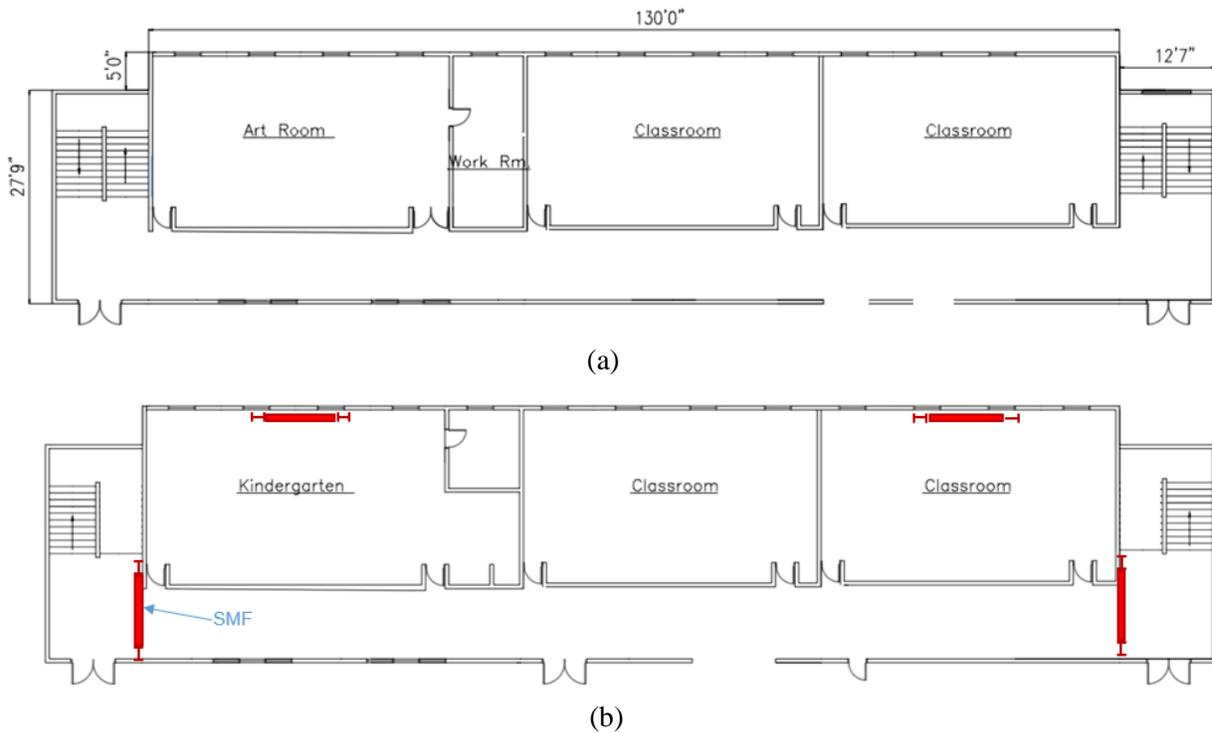
Figure 56: Proposed SMF retrofit solution for Institutional Archetype for (a) Floor 1, (b) Floor 2
