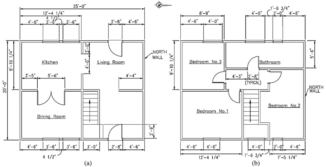
**Figure 7: Details of full-scale house (a) first floor (b) second floor**
