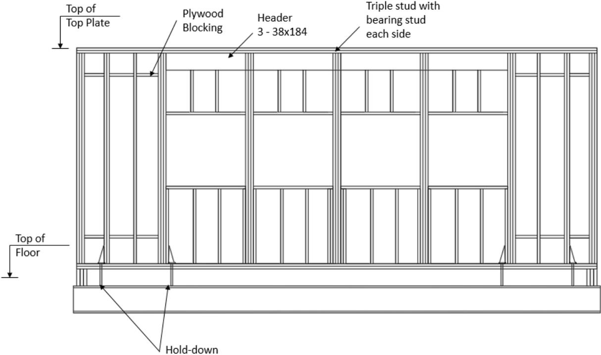
Figure E.1: Elevation – Exterior Wall Framing
