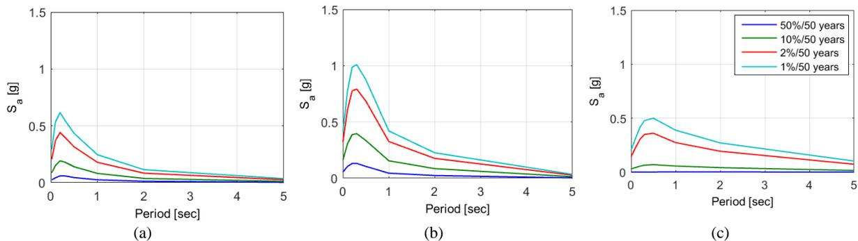
**Figure 60: Vancouver, B.C. Level 1 – 4 Spectral Acceleration (5% damping) for (a) crustal, (b) subcrustal, (c) subduction earthquakes**
