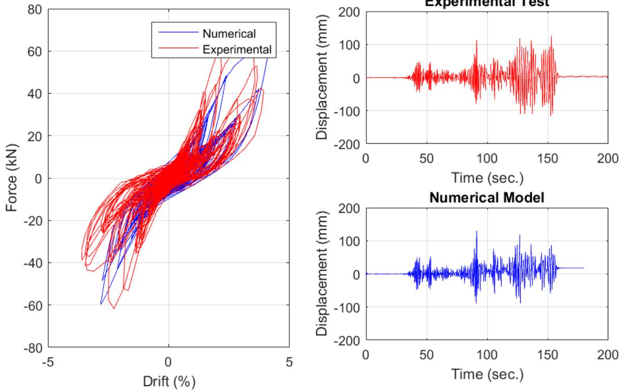
**Figure G.8: Run 2 comparison of numerical and experimental hysteretic and time-history response**
