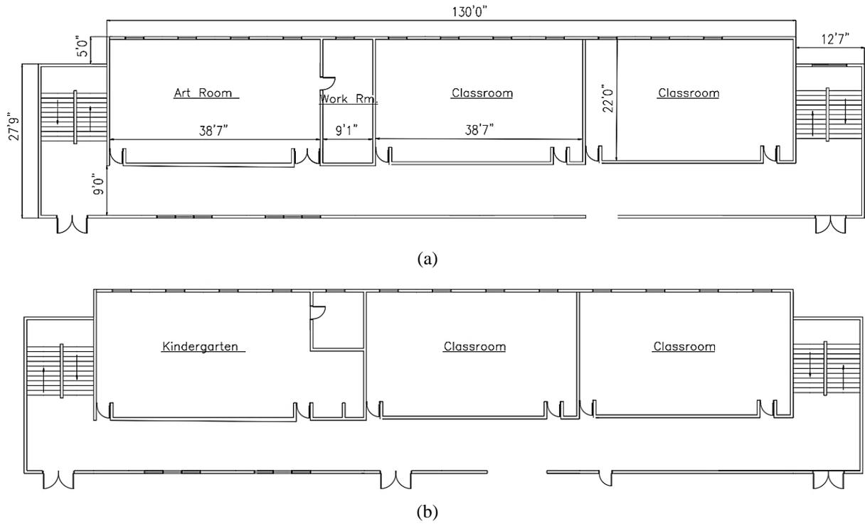
Figure 41: Plan View of Institutional Archetype: (a) second floor, (b) first floor
