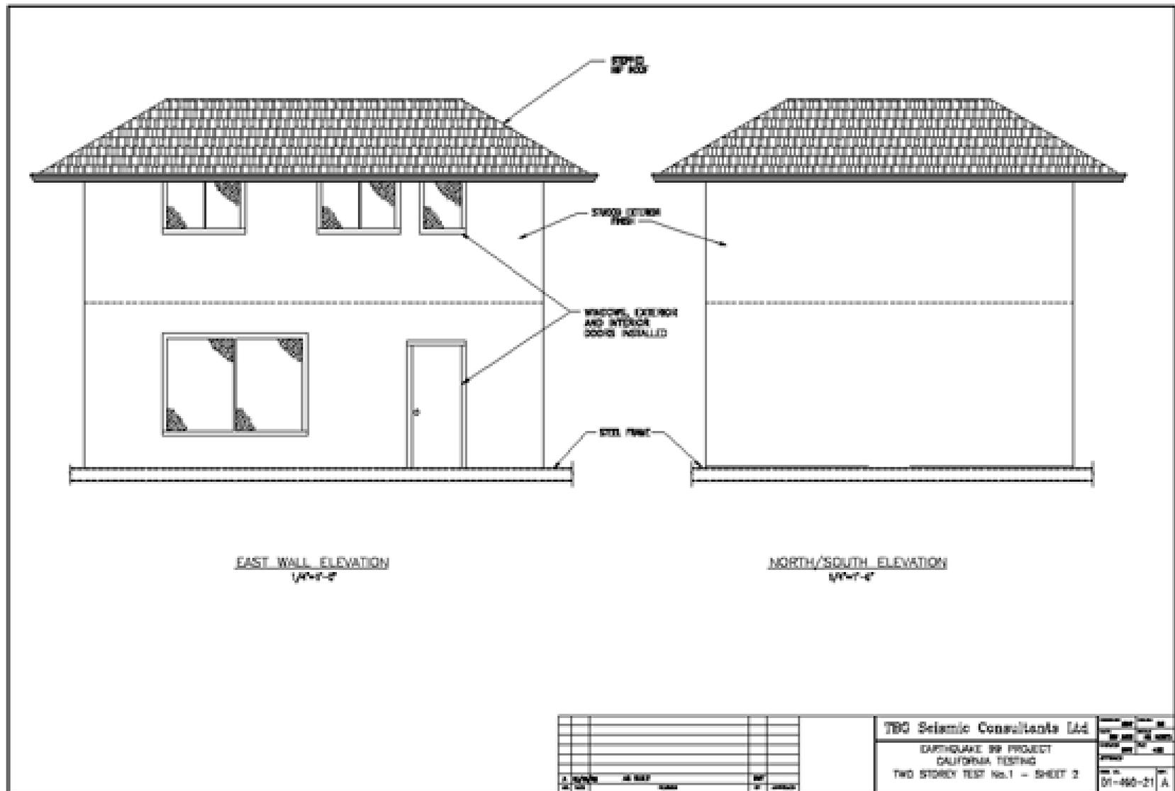
**Fig. B.1: Two-storey woodframe house elevations view**
