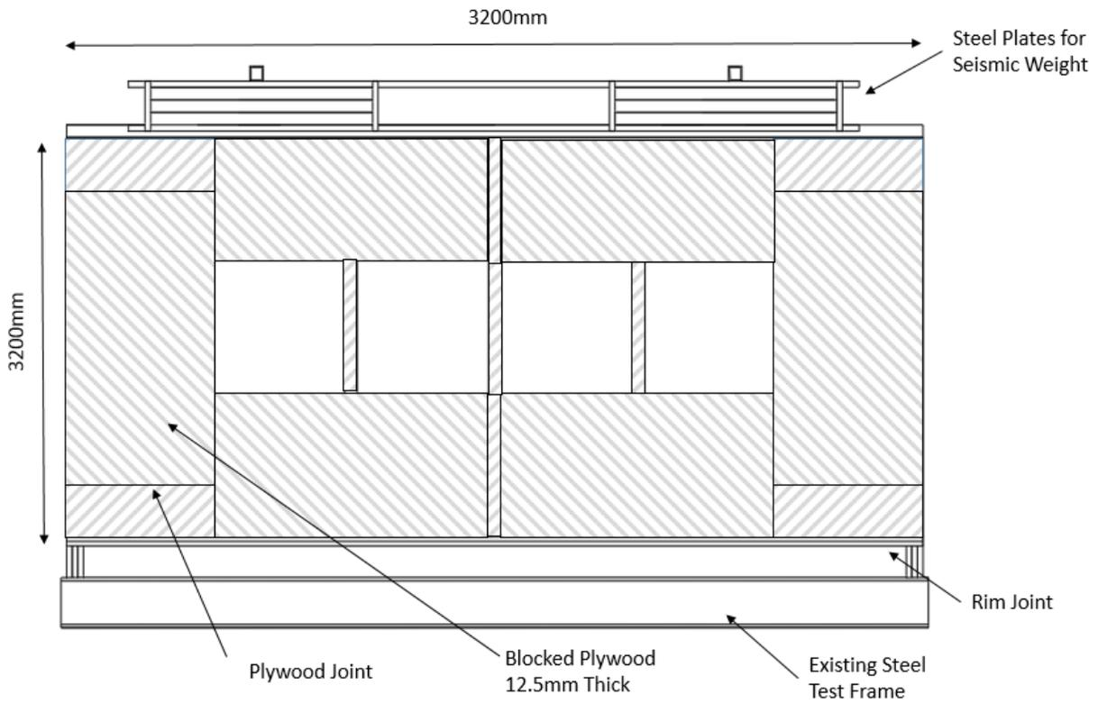
**Figure E.2: Elevation – Test Structure Exterior Wall**
