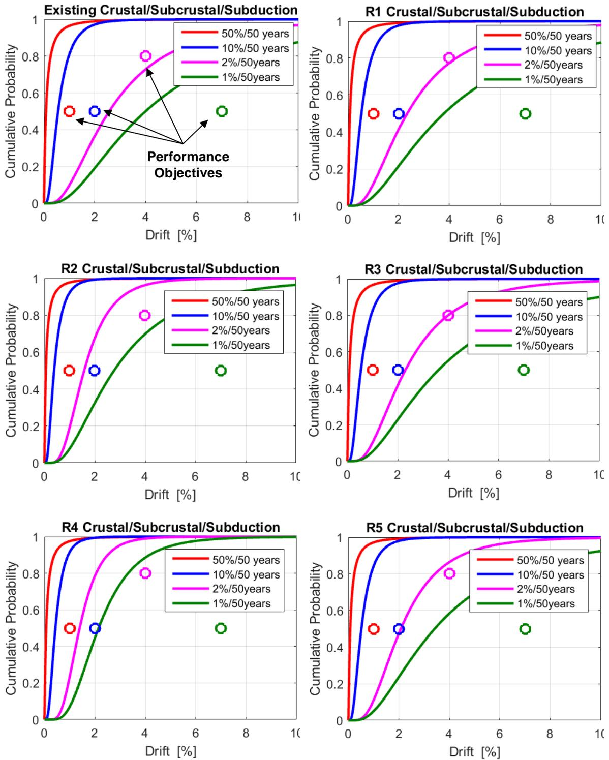
Figure 62: Peak interstorey drift distributions for the Existing Structure, Retrofit 1, Retrofit 2, Retrofit 3, Retrofit 4, Retrofit 5
