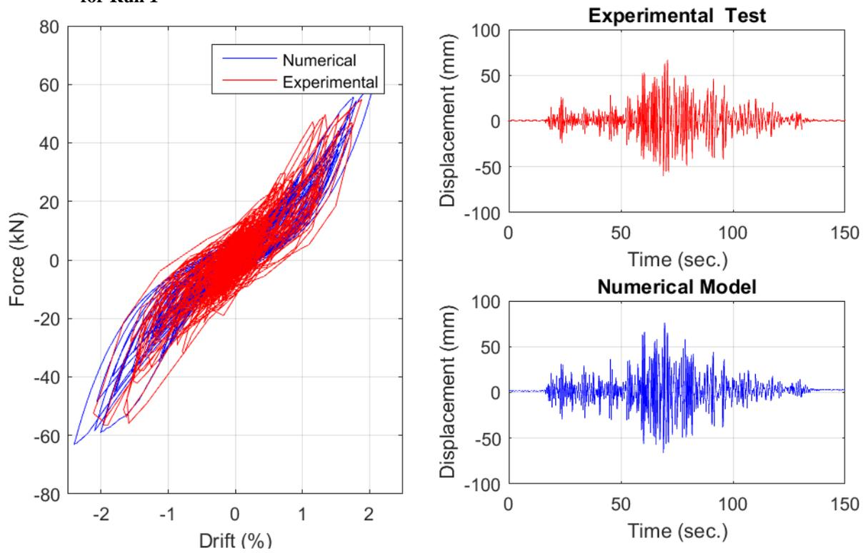
Figure 32: Detailed Numerical Model and Experimental (a) hysteresis (b) relative displacement time history for Run 2
