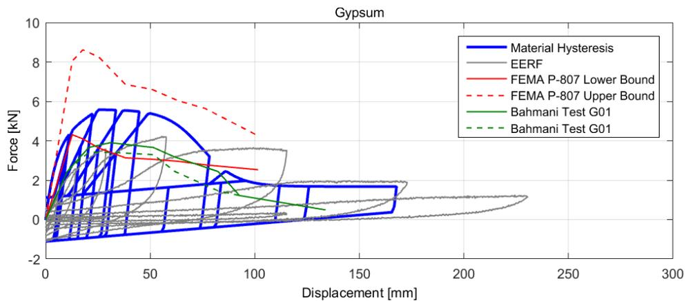
**Figure G.12: Gypsum Material Model compared to experimental data (8ft wall segment)**
