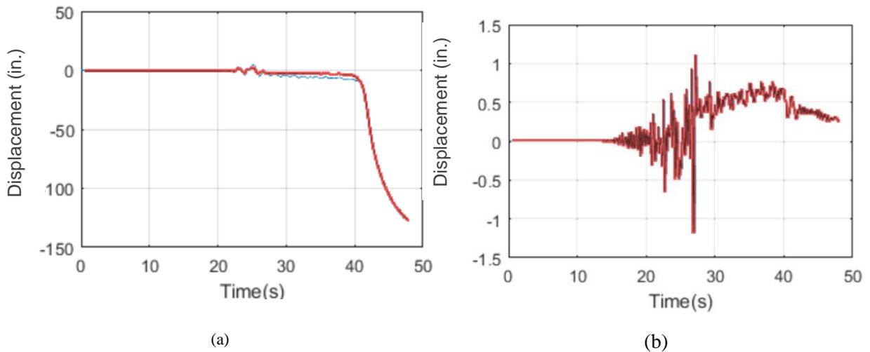
Figure 65: Time-History response of displacement at top of first storey (a) the N-S direction (b) the E-W direction
