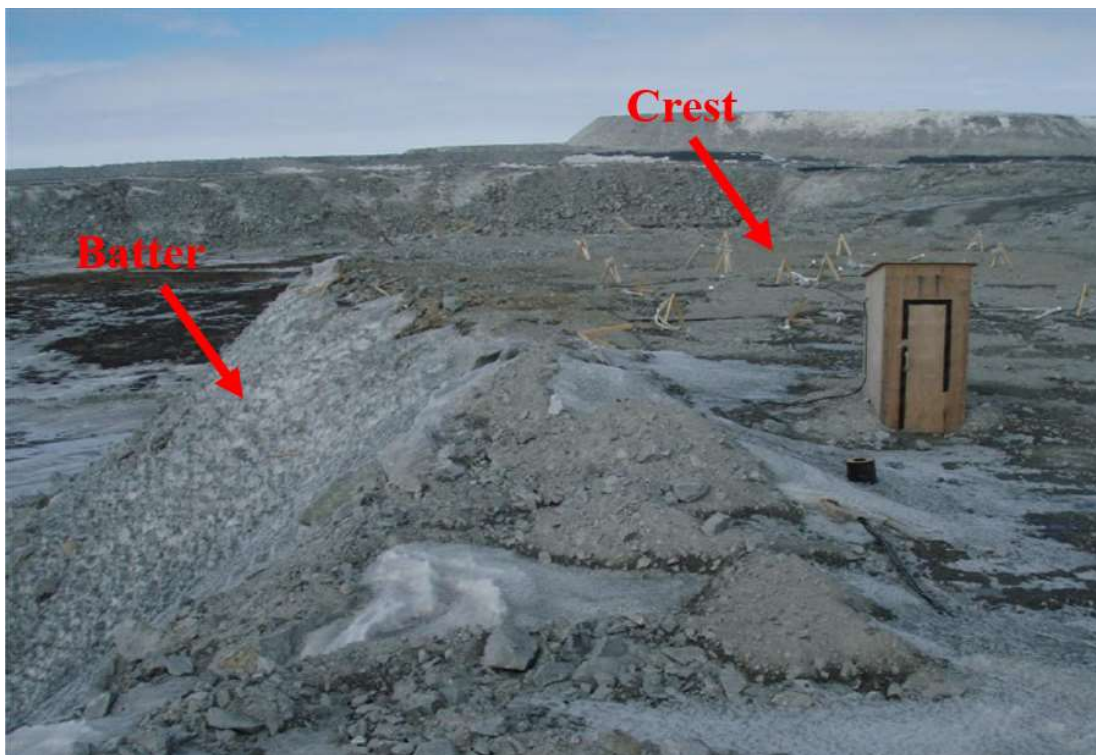
Figure 3.2. Photo showing the distribution of snow on the Type I test pile, March 16, 2008. Snow has mostly been removed from the crest and has accumulated on the batters (West batter shown). From: Neuner, 2009.
