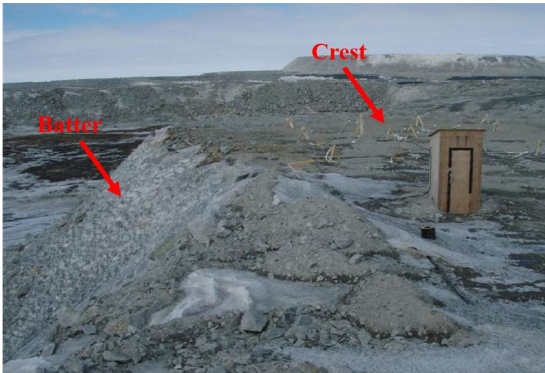
Figure 2.2. Photo showing the distribution of snow on the Type I test pile, March 16, 2008. Snow has mostly been removed from the crest and has accumulated on the batters (West batter shown). From: Neuner, 2009.
