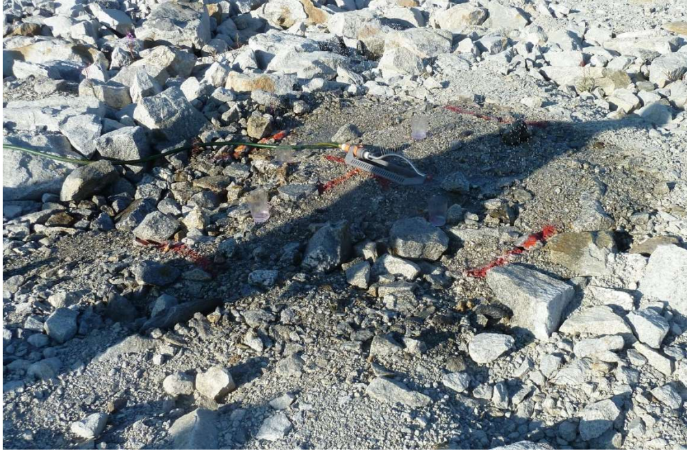
Figure E.1. Oscillating sprinkler applying a tracer event to an AZL.
