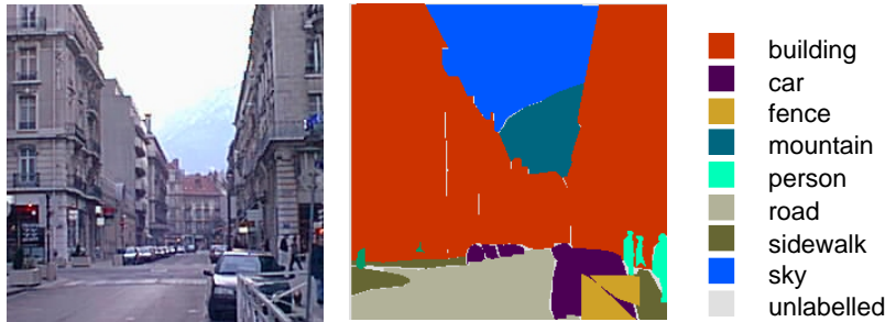
Figure 1.1: Sample output of our nonparametric scene parsing algorithm for images (Section 2) on the SIFT Flow benchmark [82].
