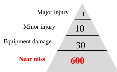
Figure 5.3: Bird's accident ratio triangle, adapted from Nichol (2012)
