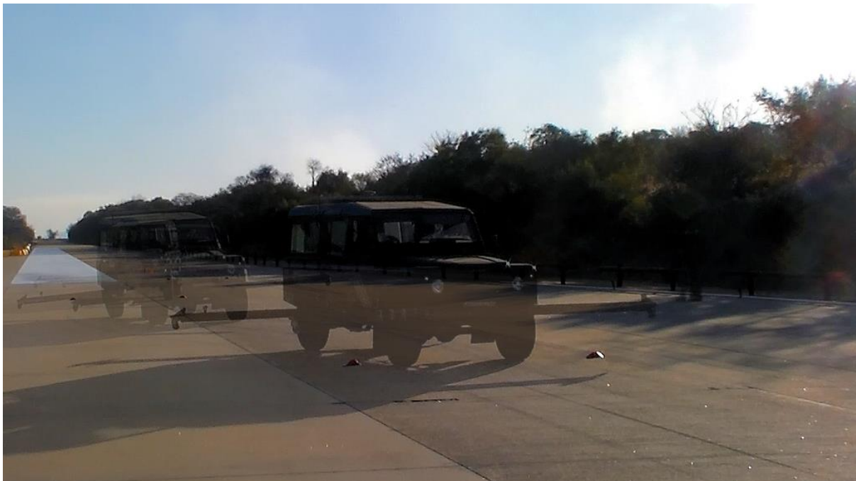
Figure 82 - ESC off (top) vs ESC on (bottom) - OA at 60km/h - Rear suspension hard
