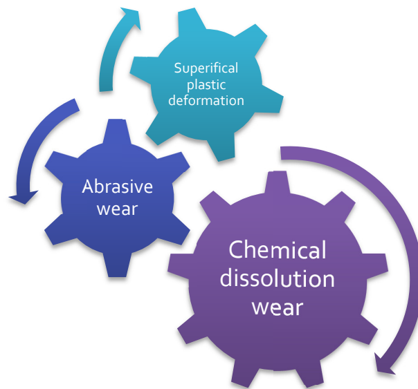
Figure 8.1. Illustration of the three main models acknowledged for describing the wear behavior of alumina-coated tools during metal cutting applications. Each model is here regarded as stand-alone models with little dependency of one another.
