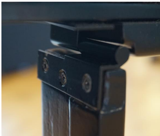
Figure 75 - Showing the hinges which fasten the legs to the frame which holds the mirror
