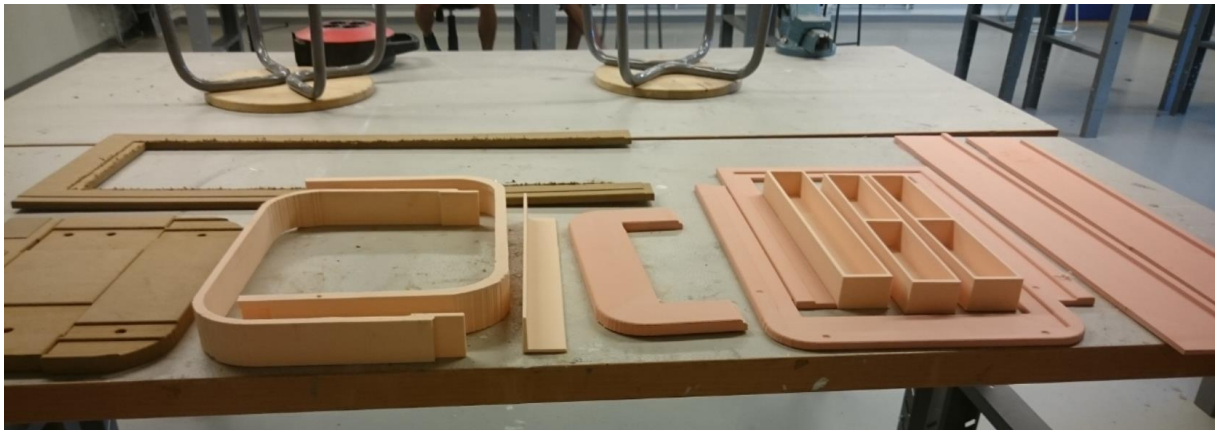
Figure 31- Showing the components that have been milled
