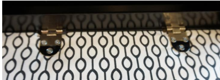
Figure 76 - Showing the hinges which mounts the ironing board to the holder
