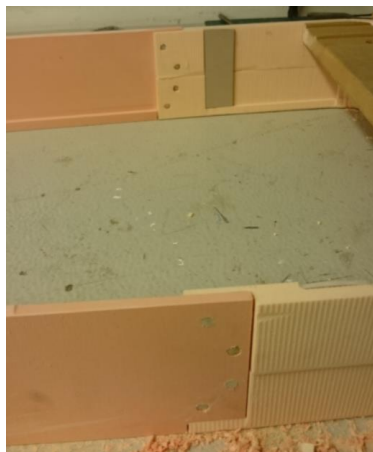
Figure 34 – Showing the step of mounting the top with the frame legs
