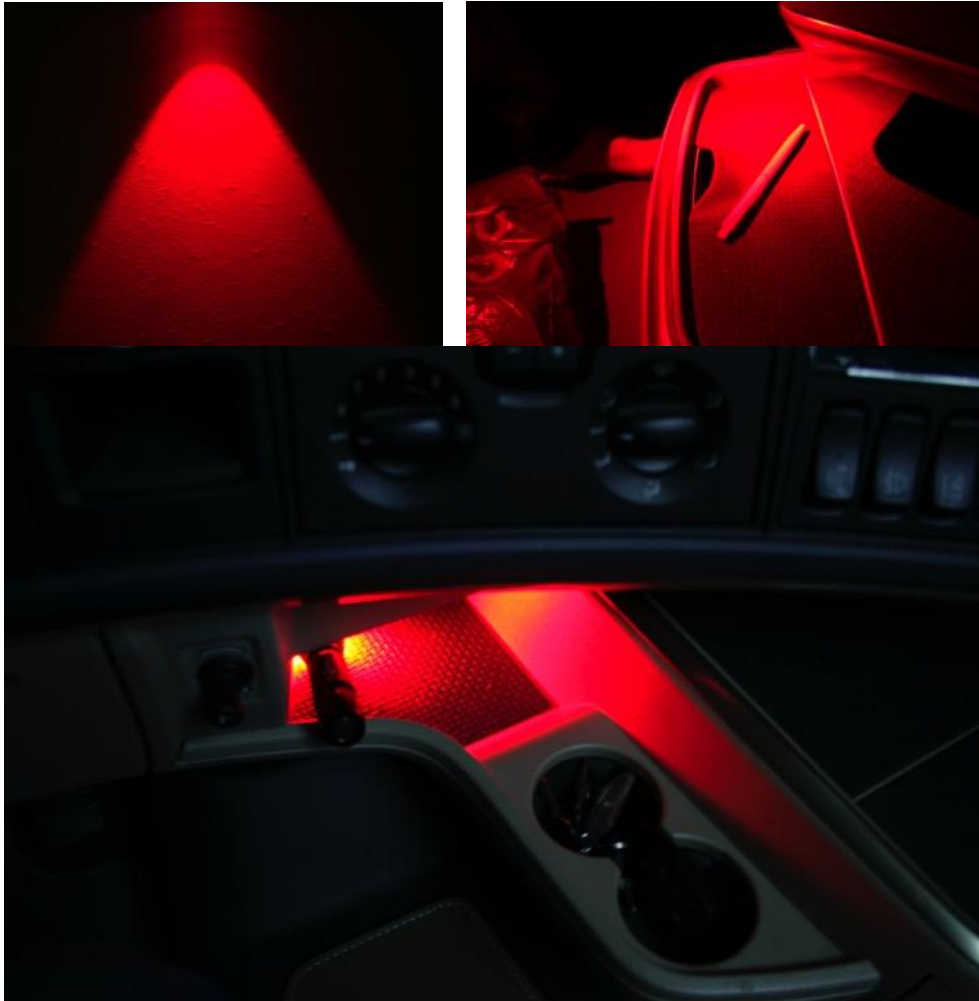
Figure 6-3, monochromatic red light is often used for ambient light while driving at night to get a general perception of the truck cab.
