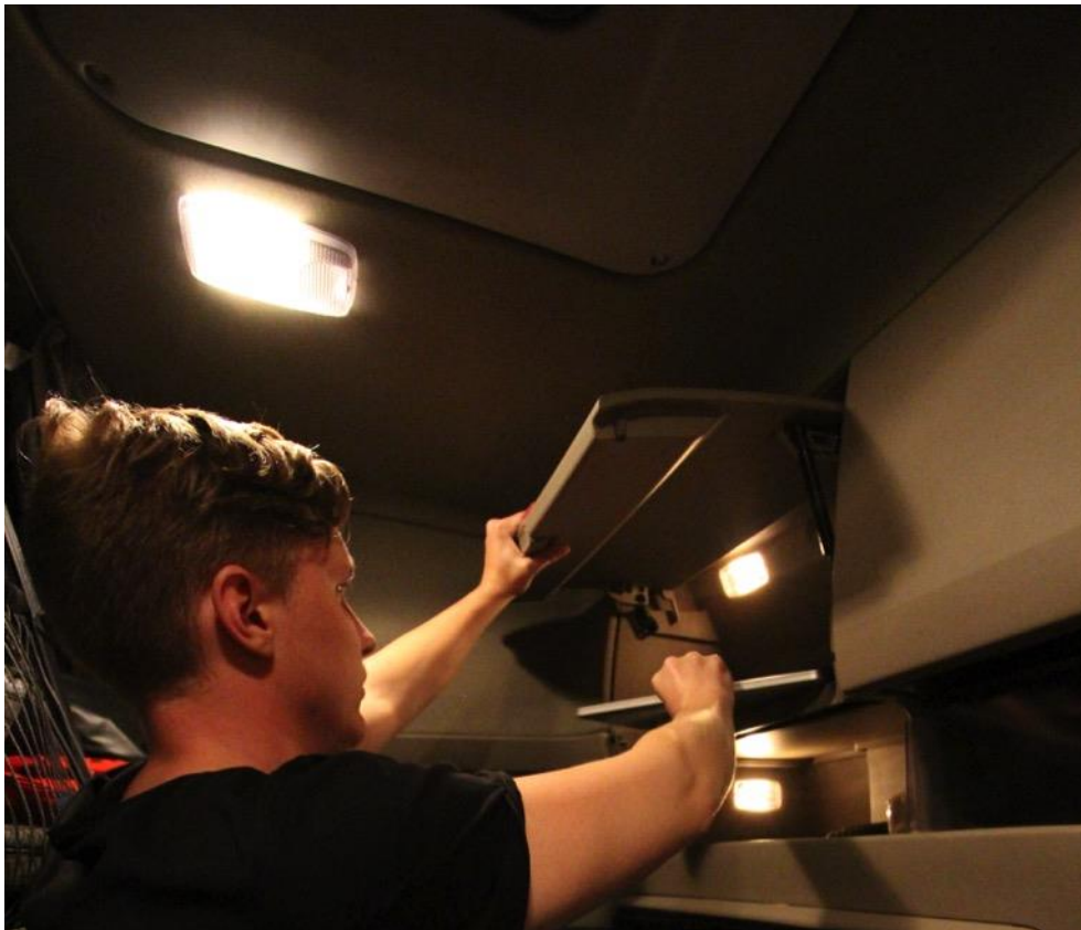
Figure 4-1, lights from storage spaces can have a glaring effect.
