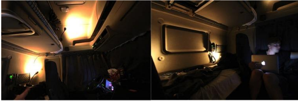
Figure 5-3, utilizing the flexibility of the reading lamps can create indirect light and cause depth and character to the interior environment of the truck cab.
