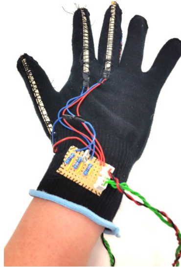
Figure 12. The upper side of the glove showing three bendable potentiometers.
