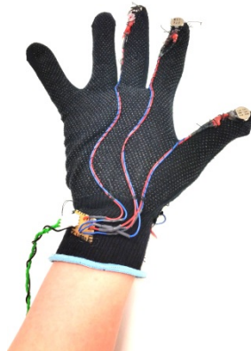
Figure 13. The palm of the glove showing three vibration motors.
