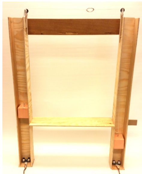
Figure 9. The final frame, consisting of two tracks on each side with blocks attached to the wire. The ultrasonic sensors are placed underneath the blocks. The glove is later on linked with the circle in the upper part of the figure.
