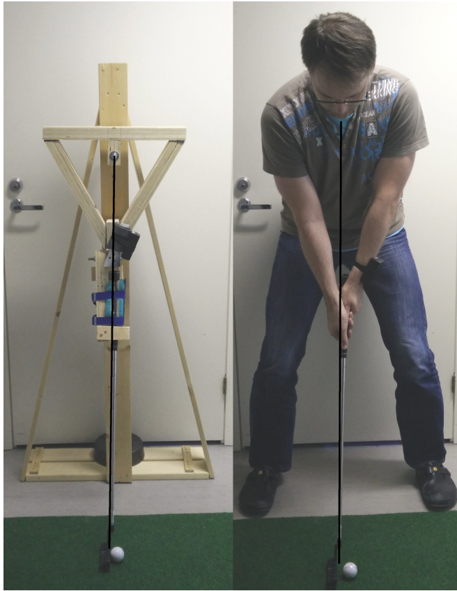
Figure 19. The putting simulation system and a human player in putting address position, with the simulated pendulum arm depicted for both.
