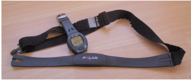
Figure 1. Polar heart rate monitor system with a sensor belt and a wrist receiver.
