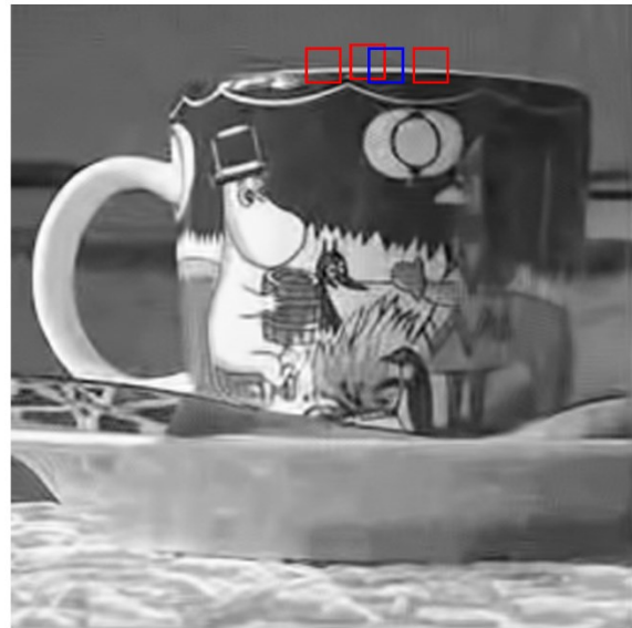
Figure 8. Processing of one block with collaborative filtering. The reference block is shown with blue borders and the nearest matching blocks with red borders. The filtered blocks are repositioned and aggregated to the output image.
