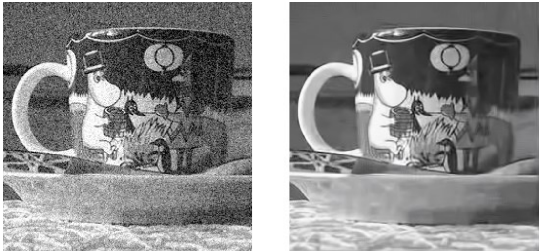
Figure 15. Noisy image with \sigma = 25 (left, PSNR 20.39 dB) and the OpenCL BM3D denoised image using the original profile (right, PSNR 28.16 dB).
