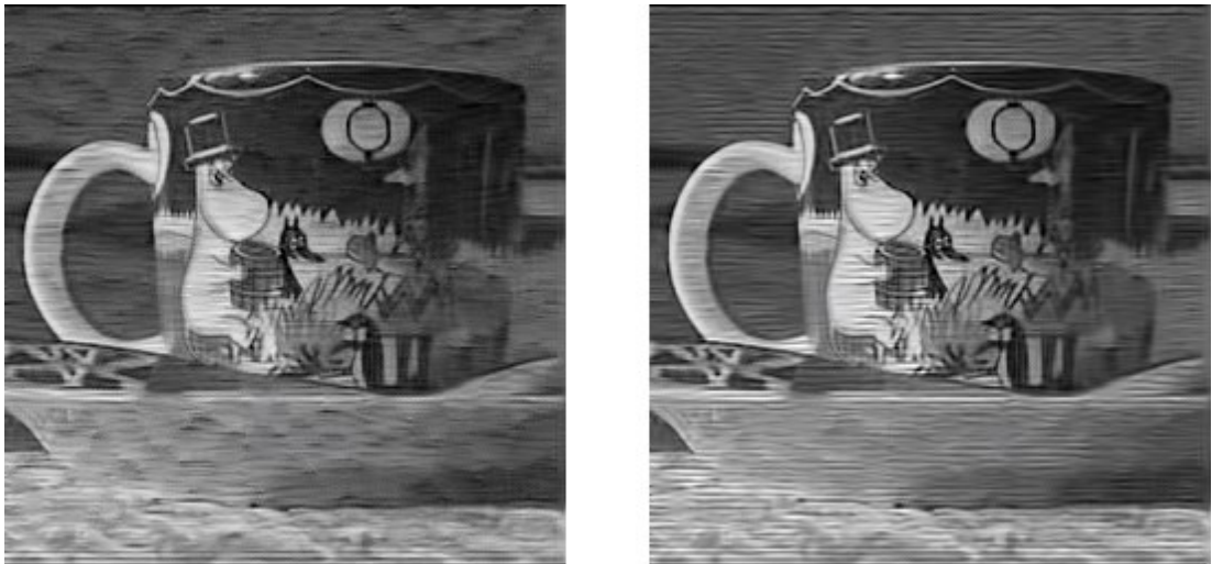
Figure 14. Computational errors while processing an image with ATI Radeon HD 5450 GPU: the basic BM3D estimate (left) and the final result (right).
