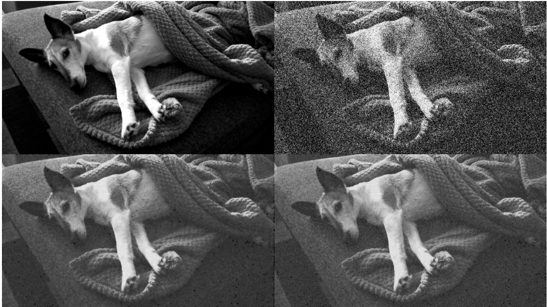
Figure 17. A 4K UHD image filtered with the OpenCL implementation: original image (top-left), noisy image with \sigma = 100 (top-right, PSNR 10.76 dB), result with modified profile after first step of BM3D filtering (bottom-left, PSNR 20.49 dB) and final result of BM3D filtering (bottom-right, PSNR 19.61 dB).
