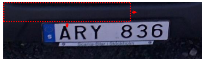
FIGURE 3.6: An illustration of how the sliding search window tests all possible locations for a license plate.
