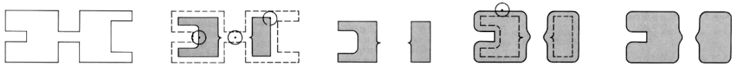
FIGURE 3.2: An illustration of the morphological closing. From left to right: original shape, erosion with a round element, result of the erosion, dilation of the eroded shape, result of the dilation.
