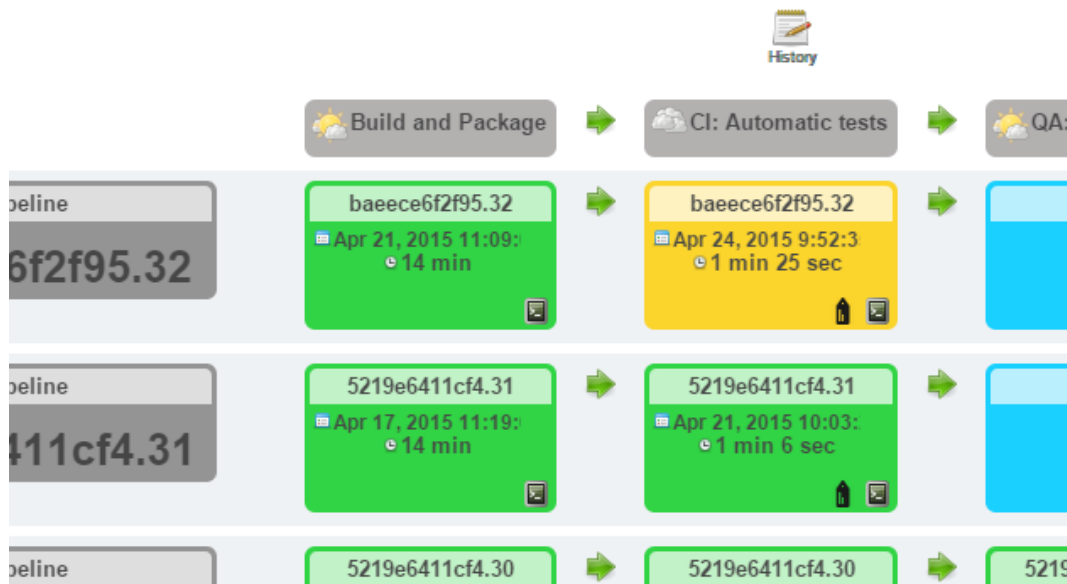
Figure 1 - The build pipeline of target_app . This is what it looks like when the tests in the CI: Automatic tests phase has found issues and therefore marked the build as unstable.
