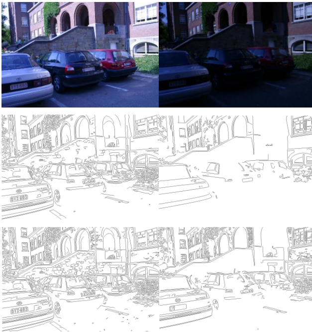
Fig. 4.8 First row: input images with illumination change. Second row: detected edges without using DT. Third row: detected edges using DT.
