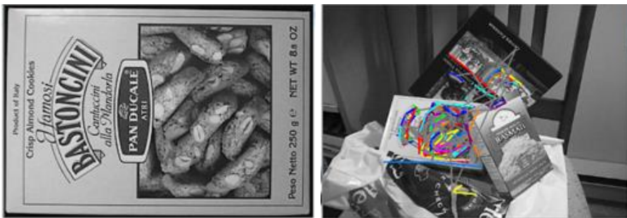
Fig. 5.4. Curve chain matching without local appearance. Left: Input image. Right: Target image and matched curves.
