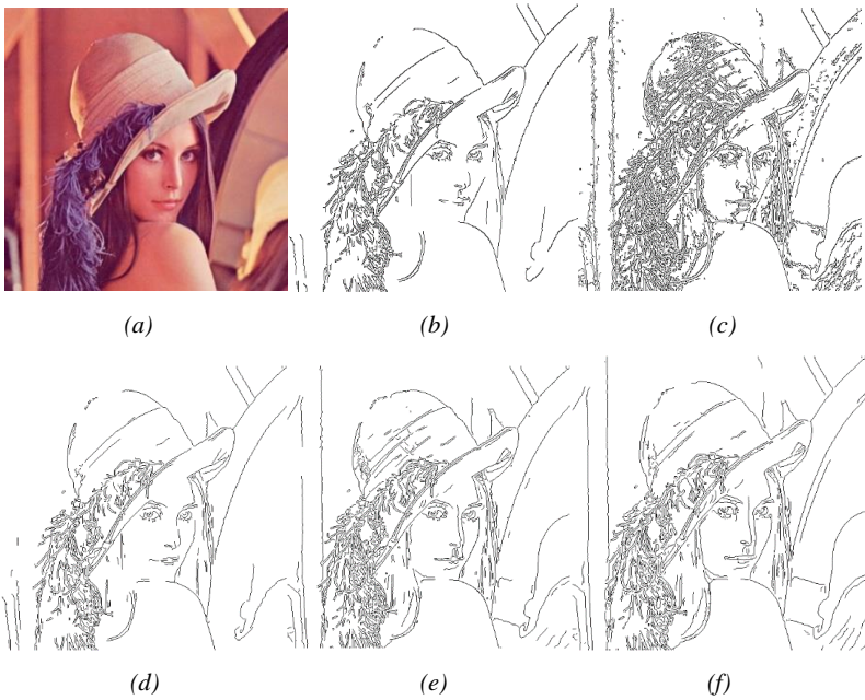
Fig. 4.9 Edge detection results. (a) ‘Lena’ image. (b) Using 3×3 Sobel filter and Canny’s scheme with high thresholds. (c) Using 3×3 Sobel filter and Canny’s scheme with low thresholds. (d) Using 3×3 COM filter and Canny’s scheme with high thresholds. (e) The proposed multi-scale method using the Sobel filter. (f) The proposed multi-scale method using the COM filter.
