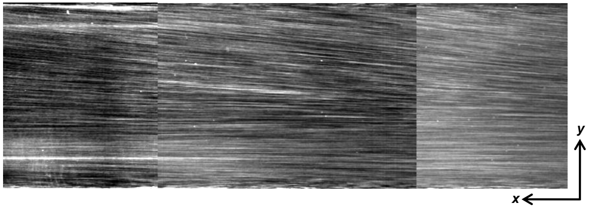
Figure 4.3 A particle pathline visualization of the flow at \Delta T = 1.9 °C in a horizontal x - y plane for 1 \text{ cm} \leq x \leq 4 \text{ cm} at z = 0.1 \text{ cm} .
